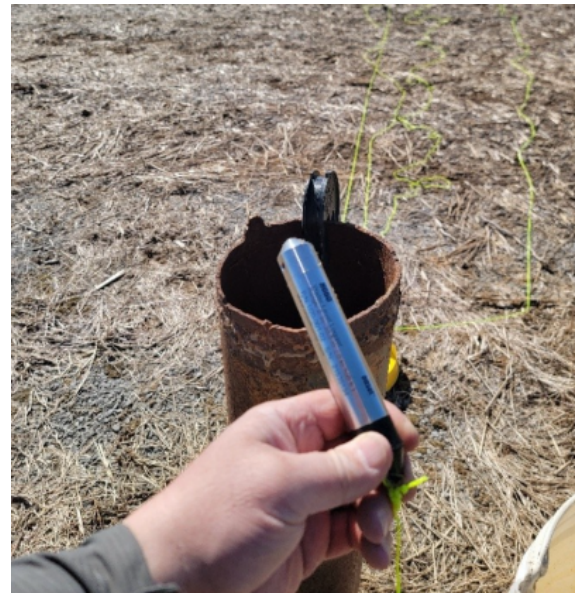
Figure 14. Glynn Beck downloading a groundwater level transducer removed from one of the monitored wells in southern Christian County.
