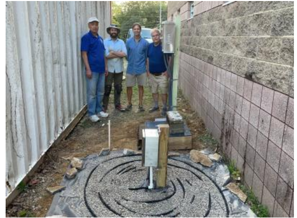
Figure 15. KGS Associate Director Zhenming Wang (left), the Earthquakes and Geophysics Team (left to right: Jon Schmidt, Seth Carpenter, and Greg Steiner ), and the completed installation of the infrasound (foreground), seismic, and strong-motion instruments at KSSMN station WIKY, Ballard County Detention Center, Wickliffe. Funding to purchase these instruments was provided by KRCEE.
