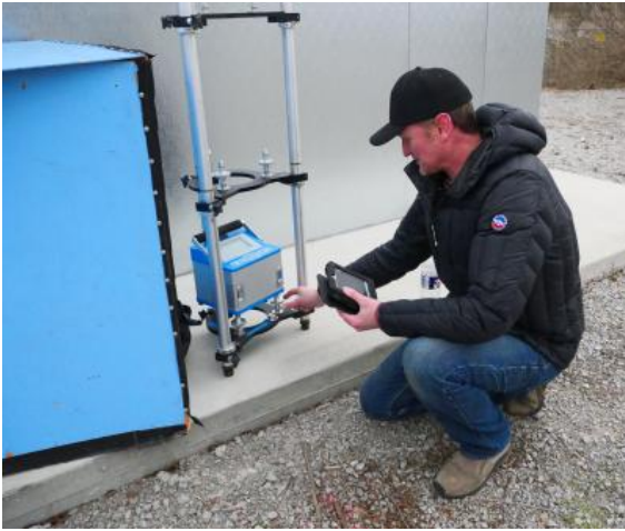
Figure 4. Jeff Kanney with the National Geodetic Survey is measuring absolute gravity for gravity modeling and determining precise surface elevations.
