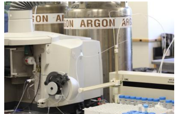
Figure 53. The Thermo Elemental ICP-OES (ion coupled argon plasma optical emission spectrometer) is utilized in the determination of rare earth element concentrations in coal ash and seam rock samples, as well as trace element levels in ground and surface water samples.
