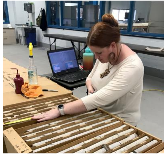
Figure 5. KGS geologist Emily Eastridge measures a section of the core as she works to describe its lithologic and secondary features.
