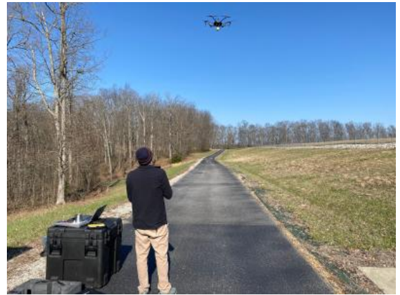
Figure 25. Matt Crawford was flying the 6-rotor UAV carrying a YellowScan Surveyor lidar laser scanner at Maxey Flats.
