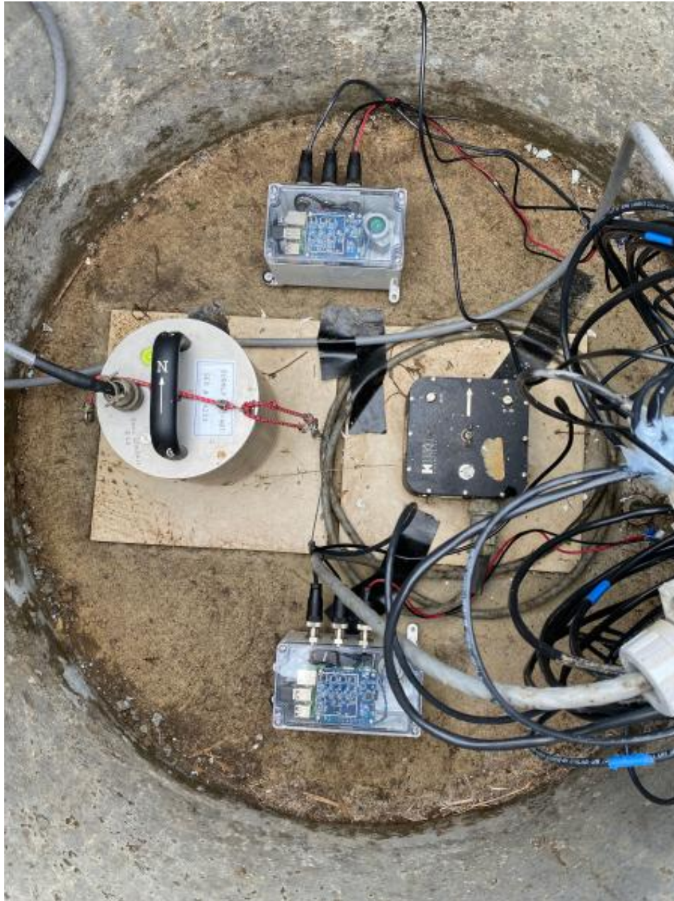
RS3D (top) and RS4D (bottom) are collocated with FBA-23 strong motion accelerometer and Guralp broadband seismometer in the instrument vault at CUSSO.
