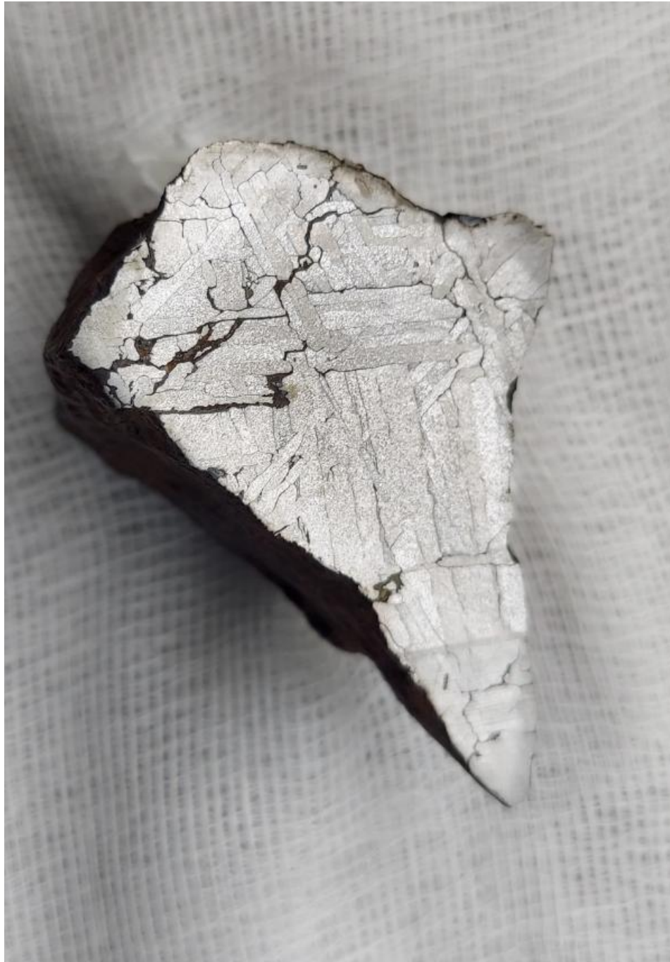
Sliced, polished, and etched section of the Handys Bend meteorite displaying Widmanstätten pattern. Photo by Ethan Davis.
