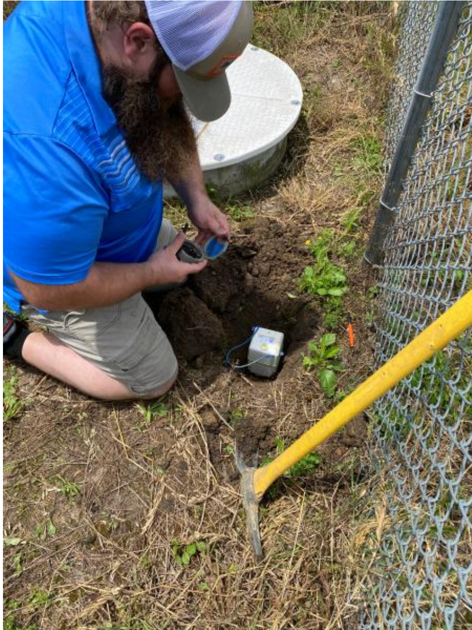
Russel Rogers, Paul Edwin Potter Intern, installing a nodal geophone at station CUSSO (photo by Zhenming Wang).
