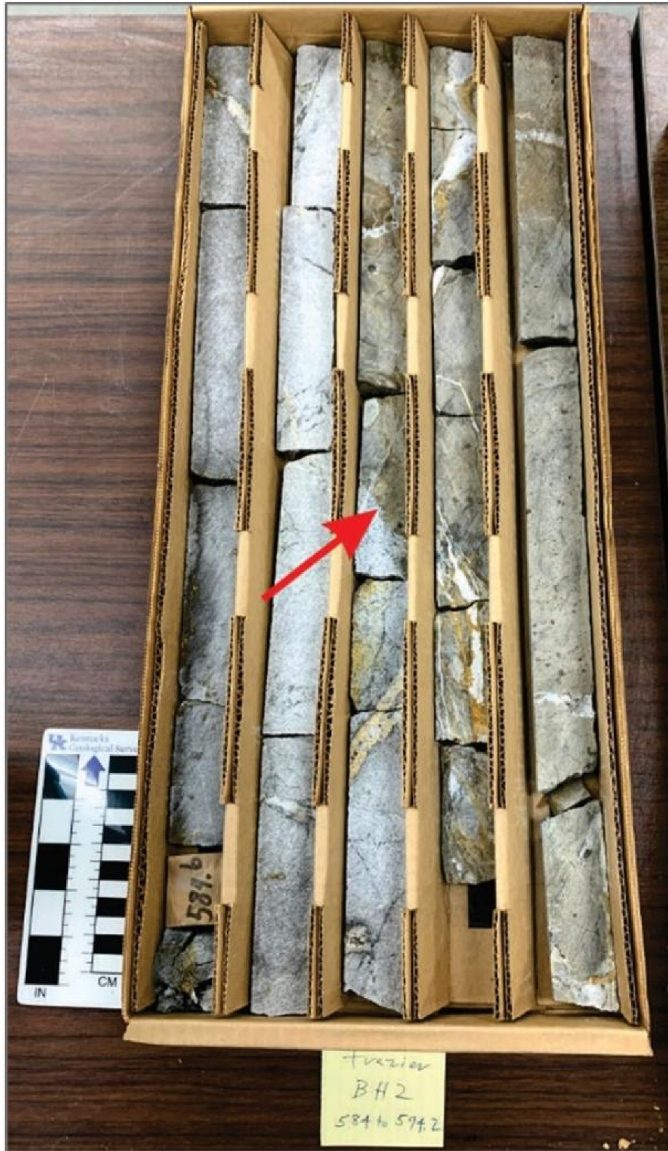
Core BH-2 from Hutson Mine, Livingston County, Kentucky (KGS call no. 1199). Red arrow points to the contact between Mississippian limestone (light gray) and the light brownish green igneous dike. The dike displays complex alteration, including cross-cutting calcite veins.
