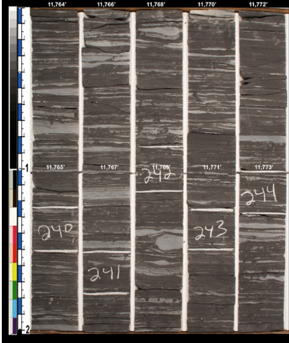
Typical Rogersville Shale core: Chesapeake Northup Law 1 well, Lawrence County, Kentucky.
