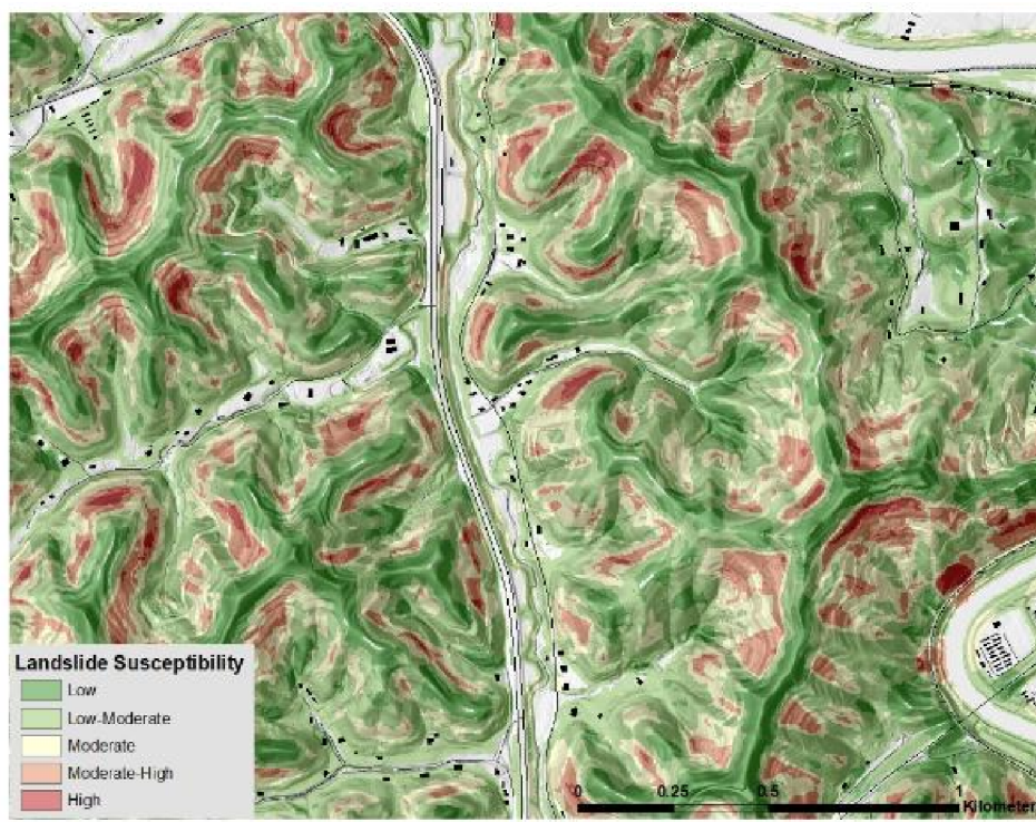
Landslide susceptibility for a part of Floyd County, Kentucky.
