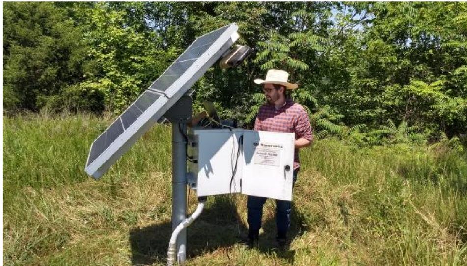
Jon Schmidt works on seismic station EK32 in Breathitt County, Kentucky.
