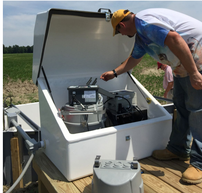
Mark Akland of the UK Department of Plant and Soil Sciences checks one of the instruments used to monitor edge-of-field water quality, soil moisture, and groundwater in the lower Green River watershed. Akland collaborates on this project with Glynn Beck .
