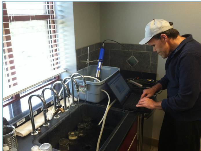
Steve Webb calibrates a data sonde to monitor changes in temperature, pH, specific conductance, and turbidity of water pumped from Head of Rough Spring to the Hardin County Water District No. 1 treatment plant near Cecilia.
