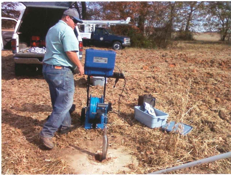
Hydrogeologist Glynn Beck uses downhole camera equipment to inspect the open borehole of an unused private water well in Oakville, as part of the evaluation for use in the Kentucky Groundwater Observation Network.
