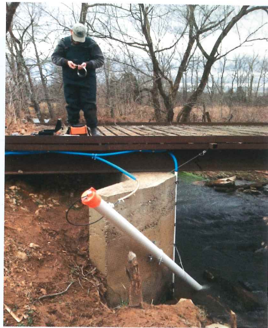
KGS hydrogeologist Steve Webb installs water-quality and water-level monitoring equipment at the Head of Rough Spring monitoring station.
