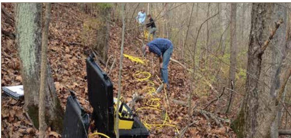
Students Clay Seckinger, Bailee Hodelka, and Clara Rucker conduct an electrical-resistivity survey for landslide characterization at the Doe Run site in Kenton County.
