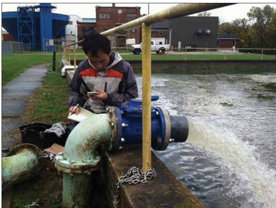
Junfeng Zhu records the rate of groundwater discharge from a municipal supply well during an aquifer test at the Elizabethtown Water Treatment Plant.
