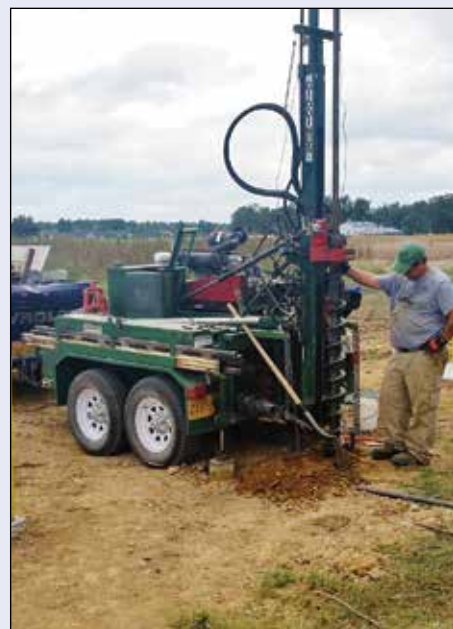
ABOVE: Scott Waninger collects a sediment core at the Murray State University Hutson School of Agriculture West Research Farm. The wells in the picture are part of the Kentucky Groundwater Monitoring Network.
