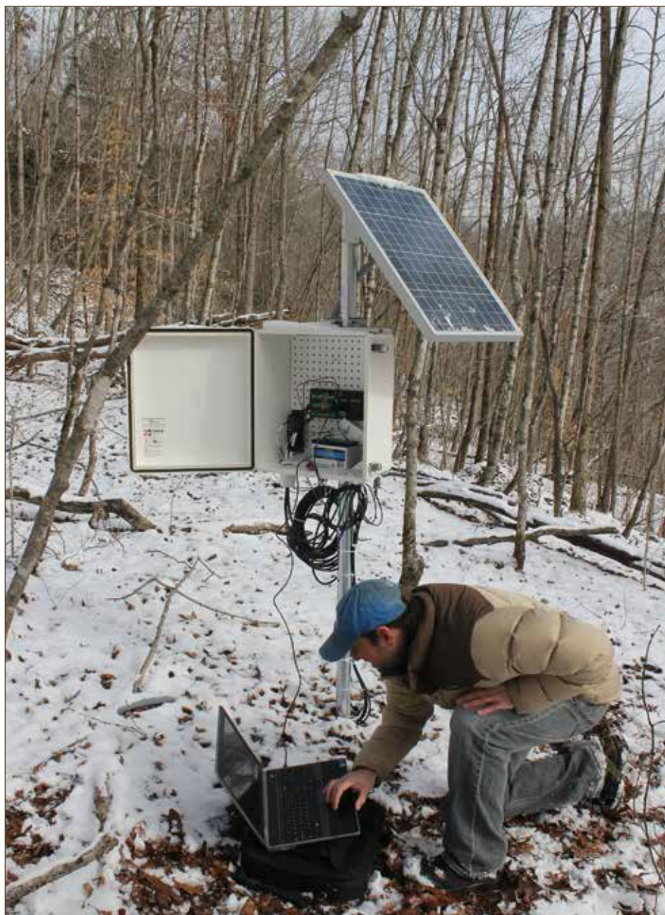
Matt Crawford downloads data from his landslide monitoring station in Pulaski County in south-central Kentucky.
