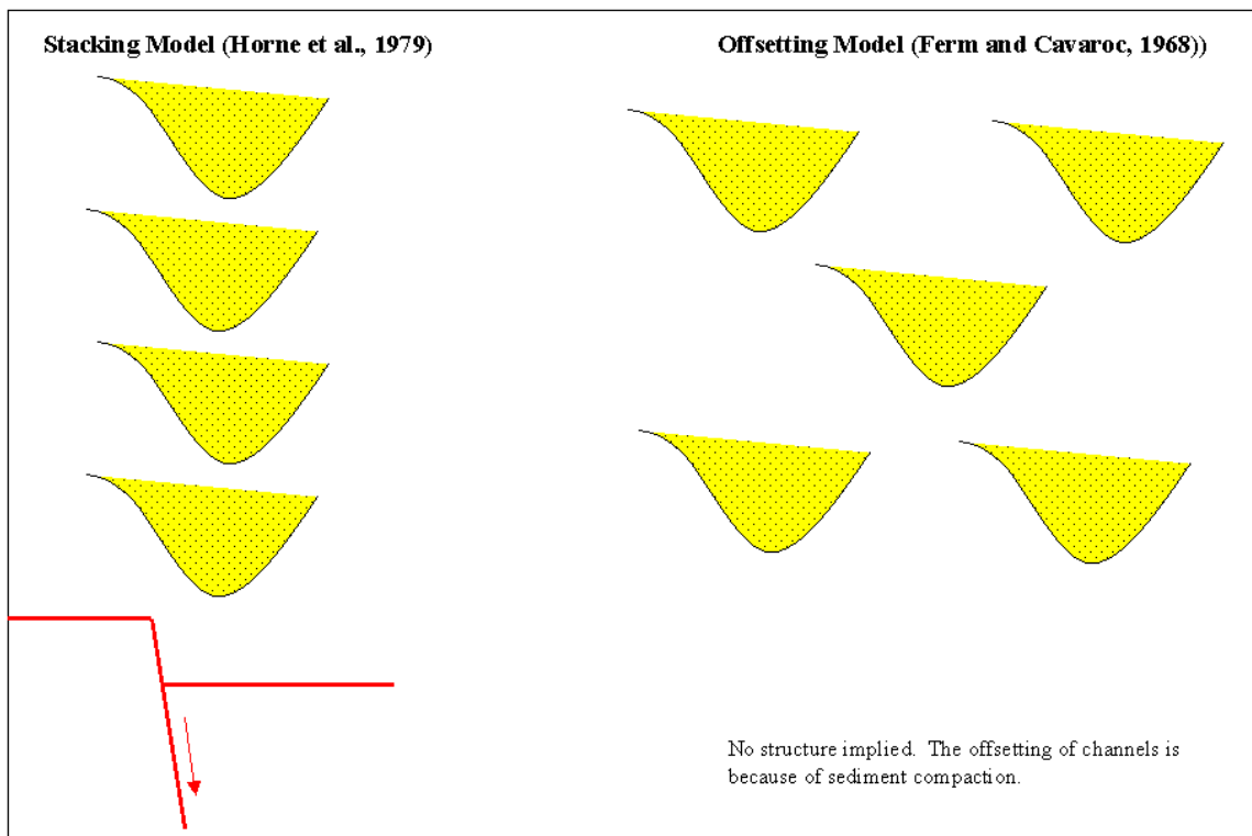
Figure 1.1: Generalized diagram showing the offsetting model (Ferm and Cavaroc, 1968) versus the stacking model (Horne, 1979).
