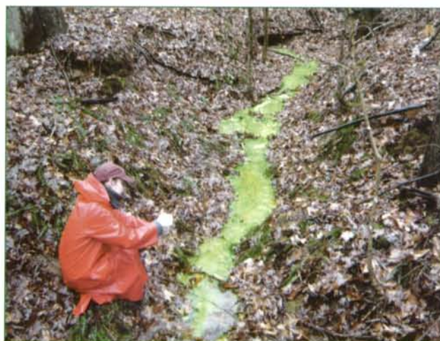
Student worker Trish Coakley pours dye into a swallow hole as a part of the project to map the groundwater basins in Radcliff.
