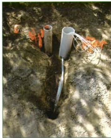
A soil gas sampler and temperature monitor set up in the Big Andy Oil Field in Wolfe County as part of Marty Parris's project to monitor the movement of gases between the air and soil at potential carbon sequestration sites.
