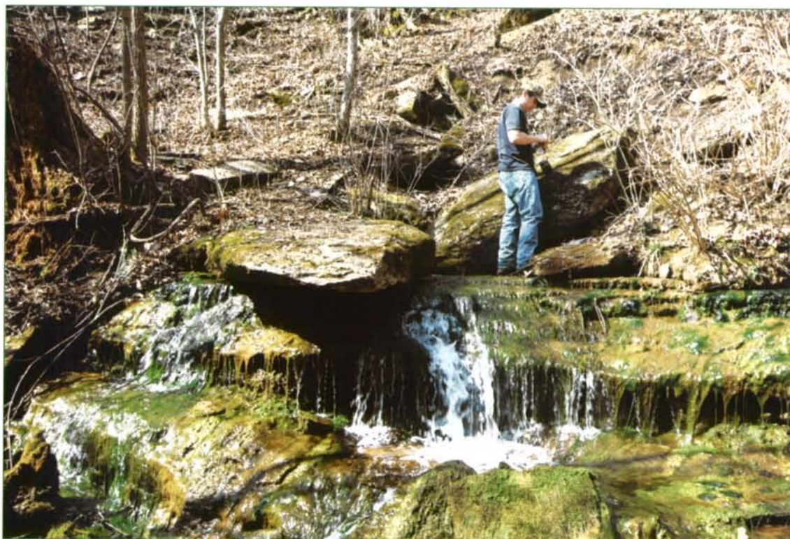
Tim Nolan, a student worker for the Water Resources Section, changes a dye receptor at Halli Spring in the Radcliff basin-mapping project.
