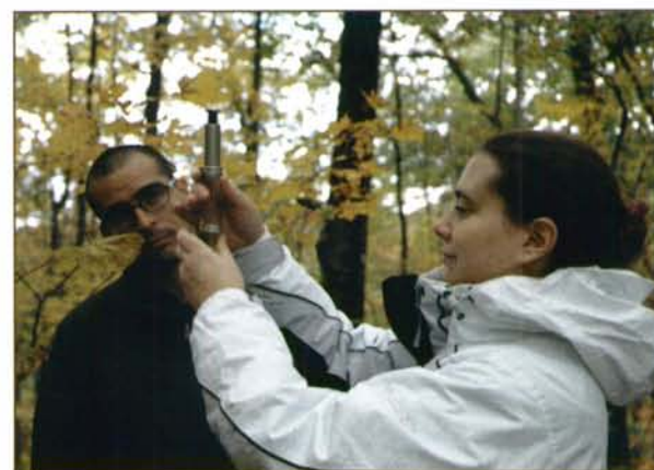
Mike Solis watches as Kathy Takacs extracts gas from a soil probe with an airtight syringe for laboratory analysis. Their field work is associated with a KGS project managed by Marty Parris to monitor existing carbon dioxide levels.
