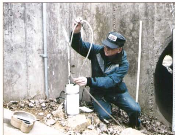
Jim Currens, of the Water Resources Section, checks a water-level recorder in a stilling well installed for the Radcliff groundwater project.
