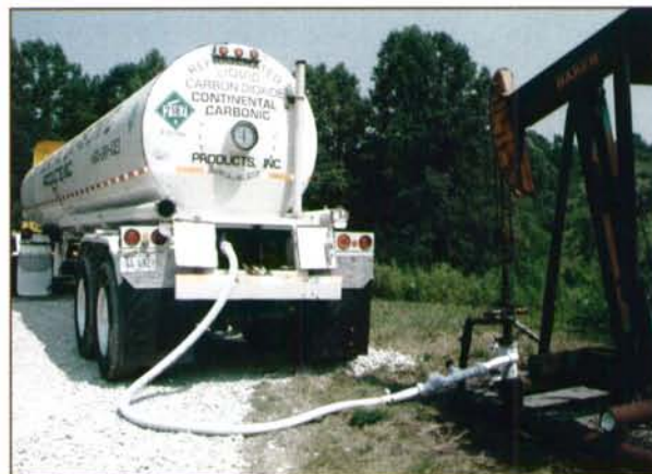
Carbon dioxide being injected into a well in Lee County, eastern Kentucky, as part of a cyclic nitrogen and CO 2 repressurization enhanced oil-recovery project.
