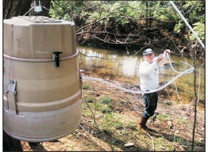
Jim Currens sets up a sampling unit on Cane Run Creek at the Kentucky Horse Park. The device automatically pumps water samples from the creek at timed intervals for laboratory analysis as part of the Cane Run watershed project.
