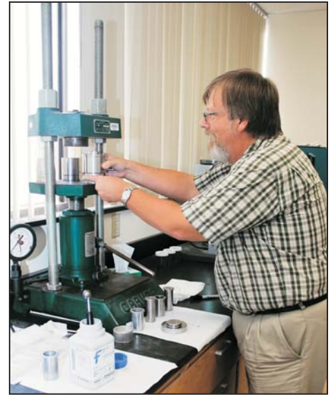
Steve Mock prepares coal samples to test them for chlorine in the lab's X-ray diffraction instrument.
