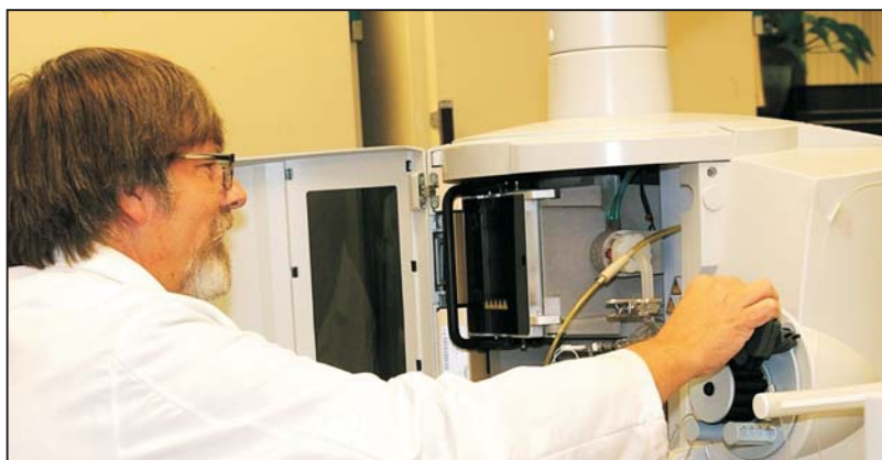
Steve Mock works with a lab instrument that analyzes metal content in water.
