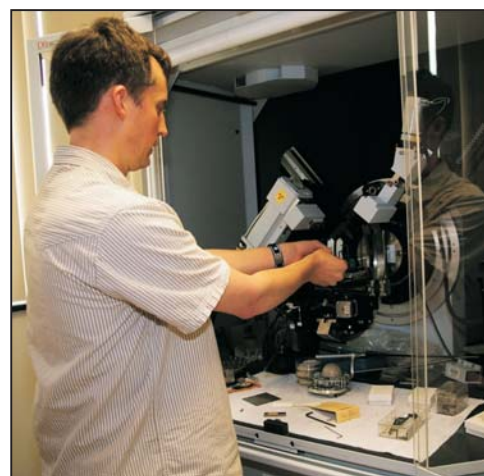
Darby Harris, a doctoral student working with University of Kentucky horticulture professor Seth DeBolt on plant cell research, places a sample for testing in the KGS laboratory's X-ray diffractometer.
