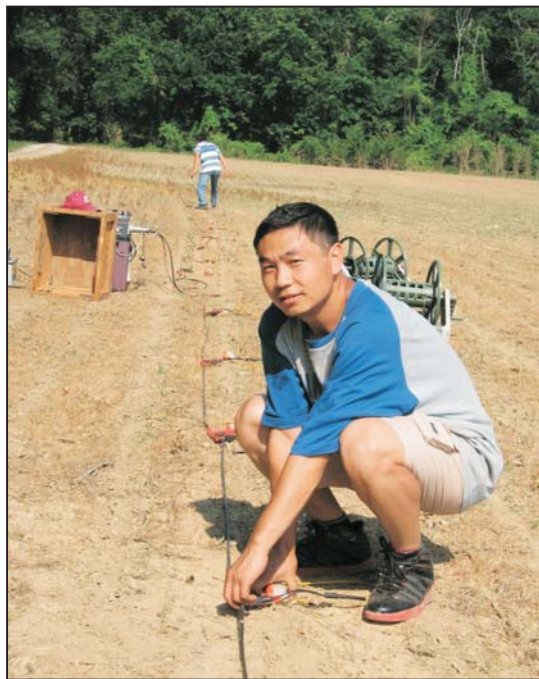
Visiting scholar Shunhua Xu couples a shear-wave geophone to the ground for a seismic velocity sounding near the Ohio River in McCracken County in a USGS-funded collaborative project between KGS and the University of Memphis.
