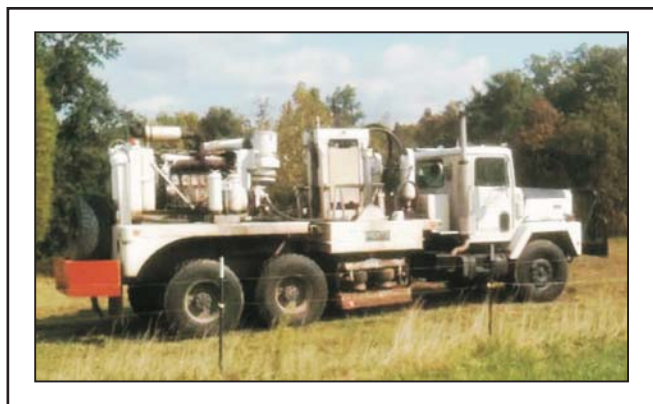
This vibrator truck was used to create the time-lapse three-dimensional vertical seismic profiles during the second phase of the Hancock County deep-sequestration test.
