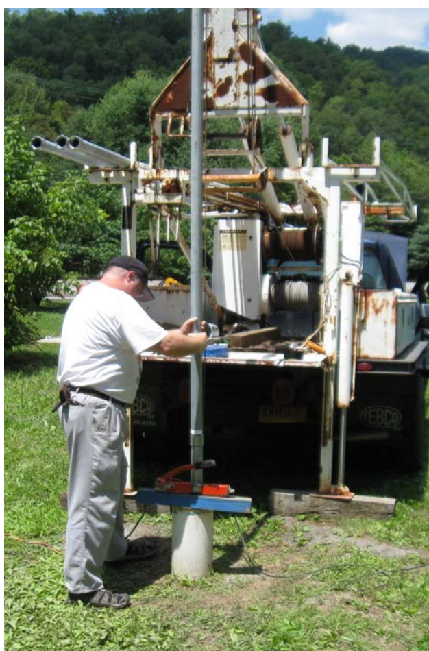
◆ Bart Davidson connects galvanized steel pipe to a water pump while performing an aquifer test at an Evarts well.
