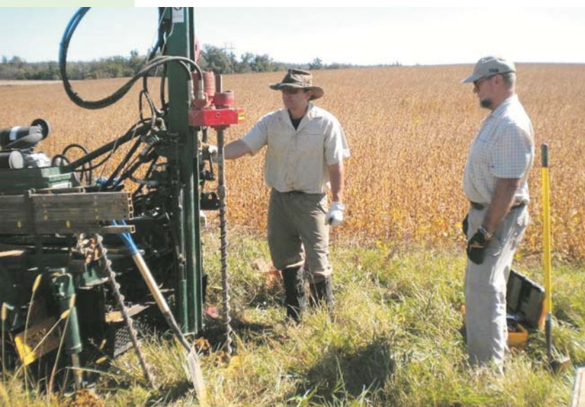
▲ Ron Counts and Mike Murphy use an augur to bore to bedrock in Henderson County as part of a mapping project.
