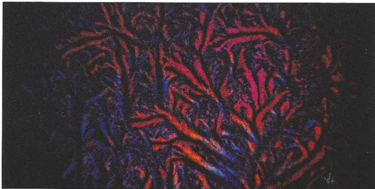
Plate 20. Photomicrograph of massive, feathery barite, from Fayette County. 25X.
