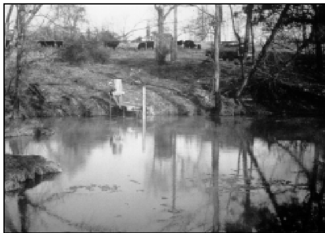
Instruments to sample water quality in the mouth of Pleasant Grove Spring. Photo by Jim Currens.
