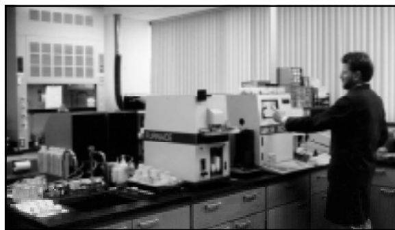
Lab personnel use this equipment to determine total sulfur and total carbon contents in coal. Photo by Collie Rulo.
