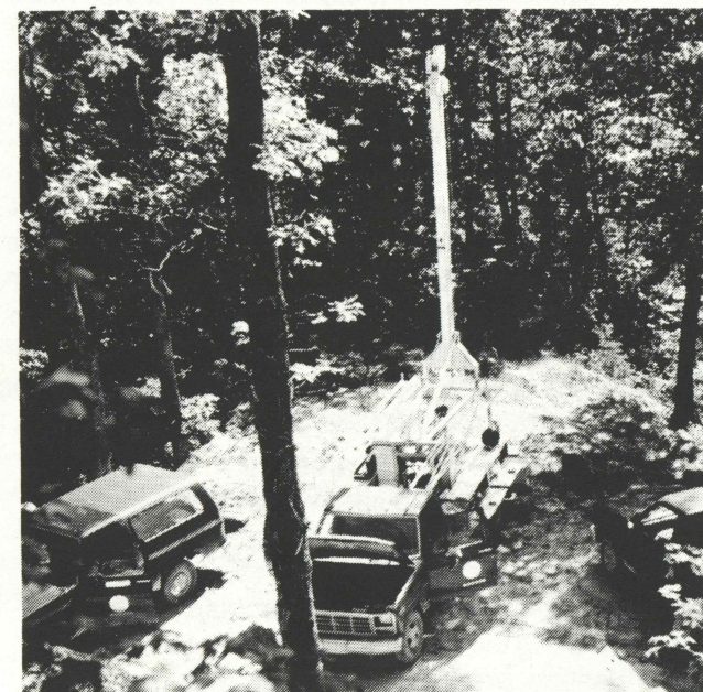
Collecting ground-water samples from monitoring wells in Robinson Forest.
