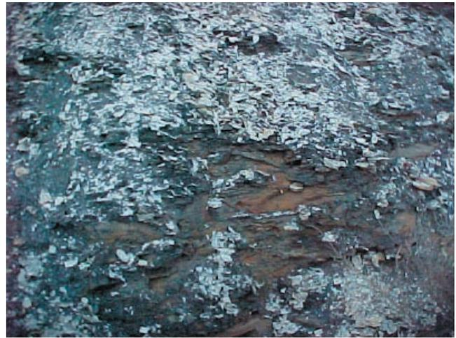
Figure 8. Secondary sulfate coating on Chattanooga Shale outcrop at the middle school.
