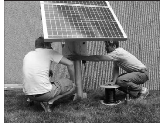
UK student Andrew Holcomb and Seth Carpenter set up of one of the new seismic instruments next to the KGS building to test its operation. The instruments rely on solar cells to charge their batteries.
