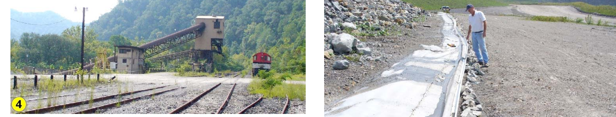
Coal Transportation This coal tipple is a loading facility for coal trucks and trains near Fishtrap Lake. Photo by Bart Davidson, Kentucky Geological Survey.
