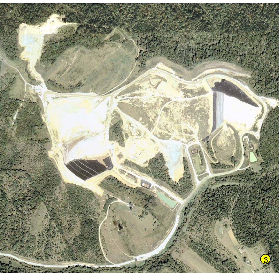
The Epperson landfill contains 1.9 million tons of nonhazardous solid waste and is permitted to accept another 3.9 million tons. A network of environmental protection systems includes a clay and synthetic liner, a leachate collection system, and a gas management system. This 2004 aerial photo was taken by the U.S. Department of Agriculture, Farm Services Administration, National Agricultural Imagery Program.
