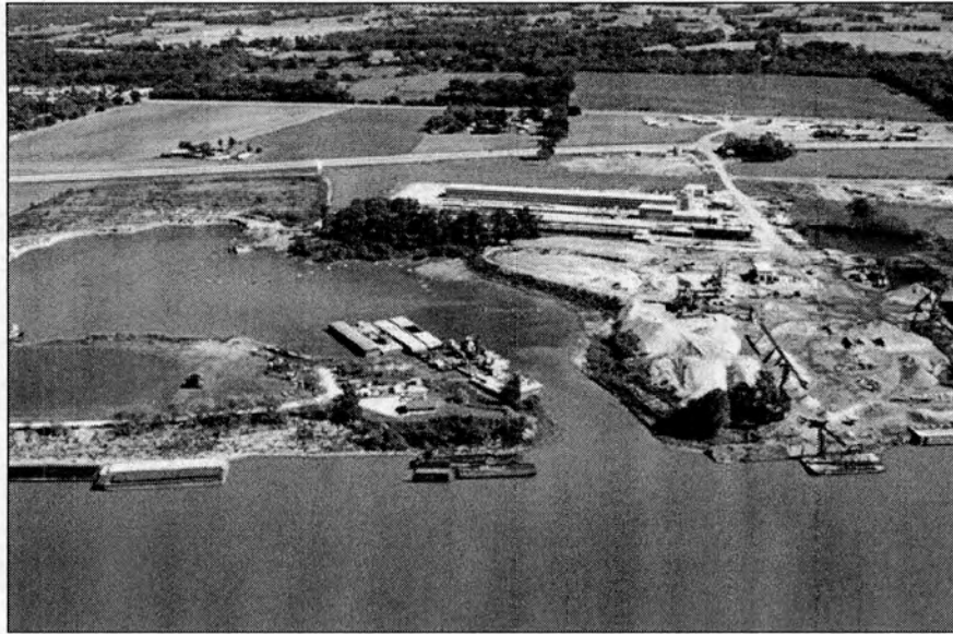
Figure 30. Aerial view of the Daviess County Sand and Gravel property, showing the dredge pond excavated into the terrace (right center) and barge loadout facilities (lower right). Photo from DCSG Web site.
