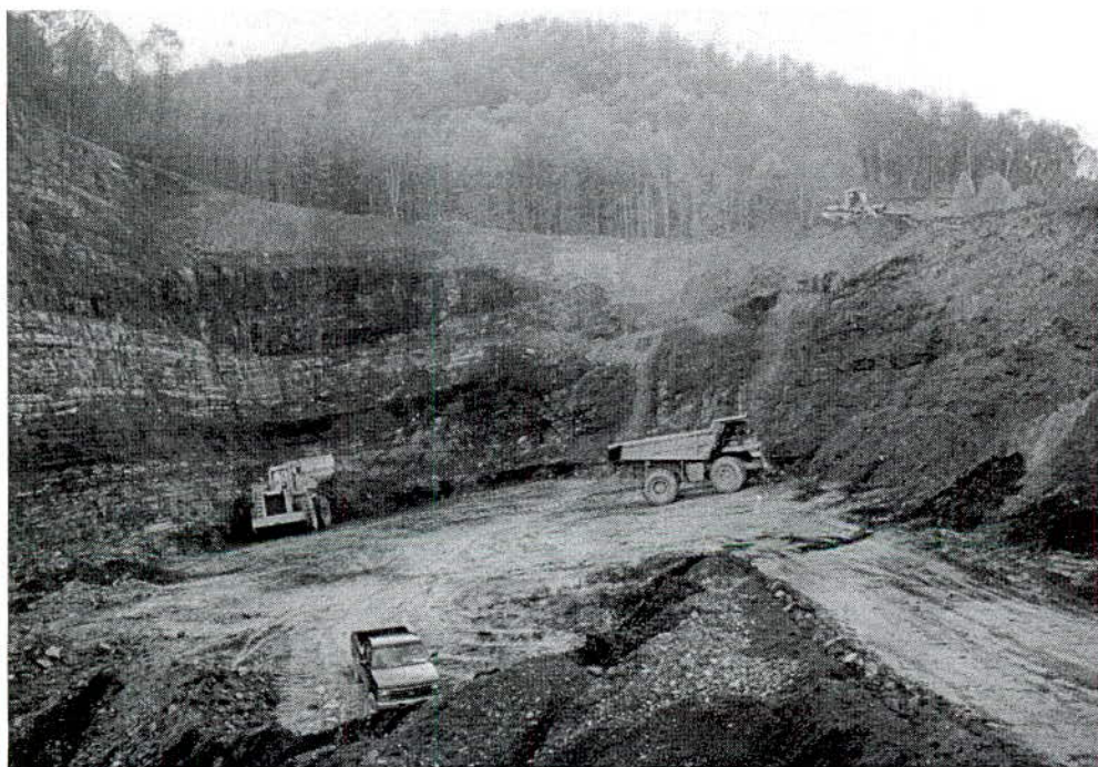
Figure 13. Surface mine pit on southwest side of the Middlesboro Basin. The coal rolled over steeply into the hillside.
