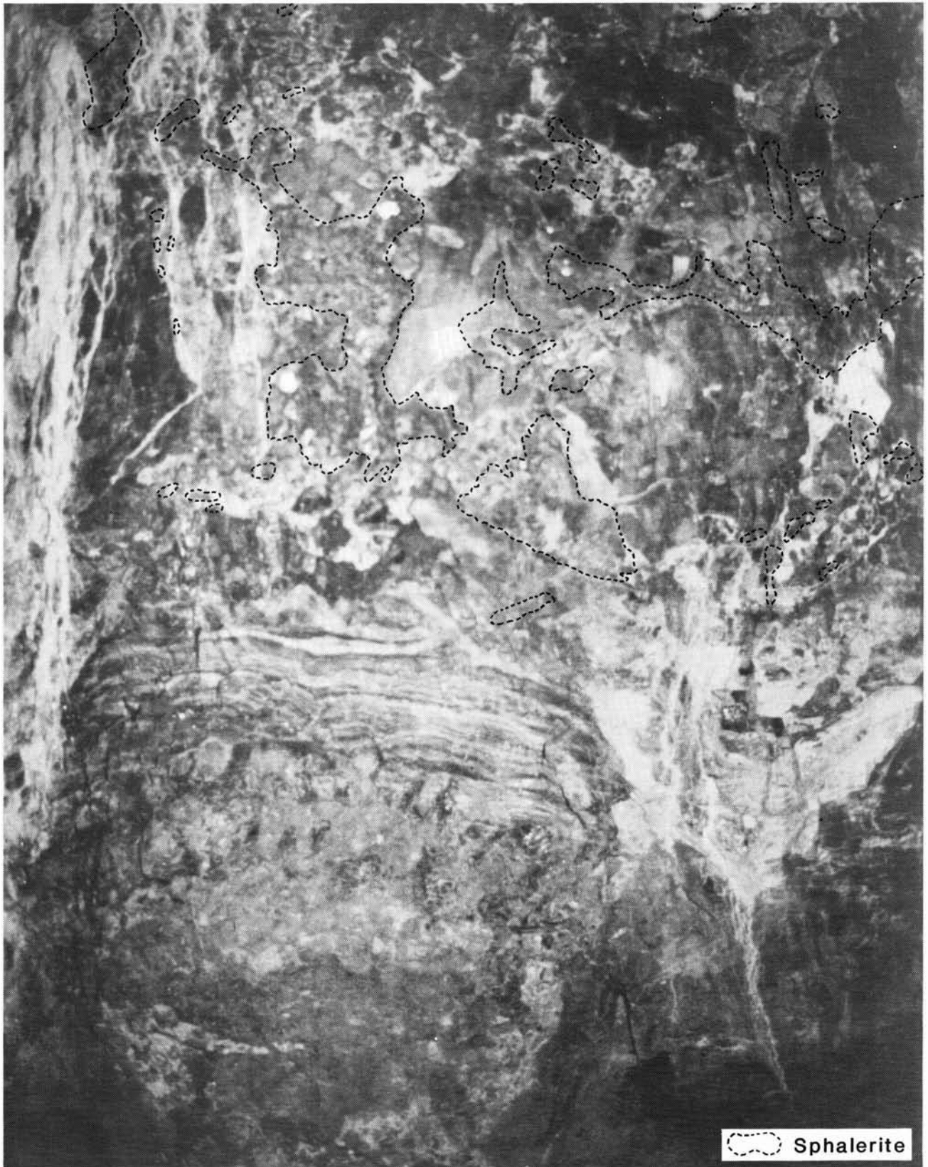
Figure 8. Mine face in the Burkesville exploration shaft exhibiting columnar stromatolites, zinc mineralization, and brecciation. (Photograph courtesy of Peter Price.)
