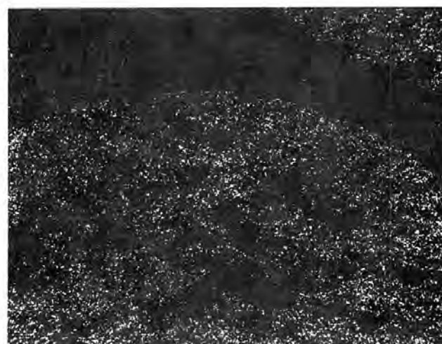
Figure 15. Cross-sectional views of alumina pellet with molybdena concentrated on surface, using scanning electron microscope. (A) Molybdena. (B) Aluminum.
