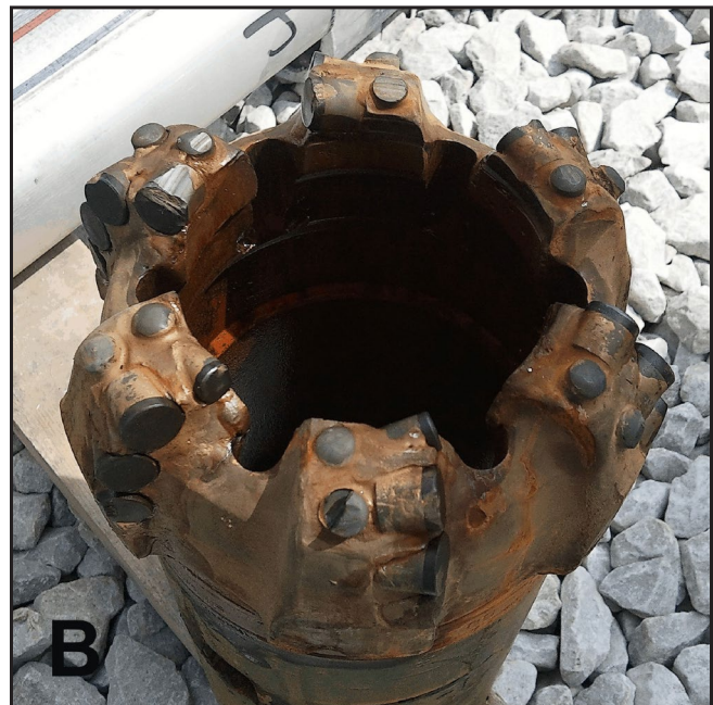
Figure 16. Polycrystalline diamond-cutter core bits used to drill the No. 1 Hanson Aggregates well. (A) A new bit (left), a gage to determine bit wear (center), and core catcher (right) to keep a core inside its aluminum sleeve for recovery. (B) A well-worn core bit after cutting several cores.
