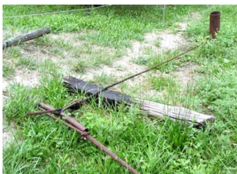
Figure 33. Turning corners. Another method of turning corners is to anchor the drive cable to a post with a short length of cable.
