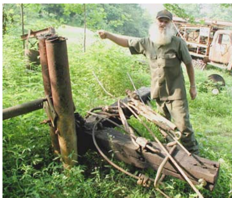
Figure 32. Swing post. A "swing post" (left) is used to turn corners on the cable-driven central power system. Cables are attached to the wooden arms that pivot about the vertical post. When everything is hooked to the cable system, 26 wells and the vacuum pump are all powered by the single 10-horsepower electric motor.
