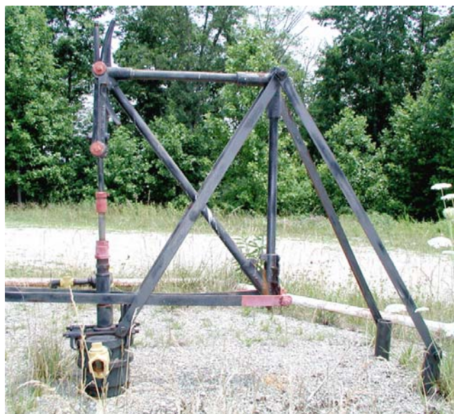
Figure 34. Jones Jack. A Jones jack was often used to lift the crude oil. A cable or rod line was attached to the base (red shackle) below the apex of the support tripod. As the cable pulled it, the arms pivoted at the apex, lifting the rods. Downhole, a ball valve assembly controlled the flow of oil.
