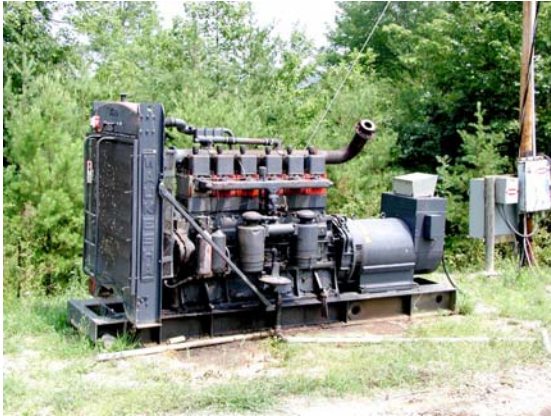
Figure 39. Generator and gas separator tank for power generation from produced natural gas.
