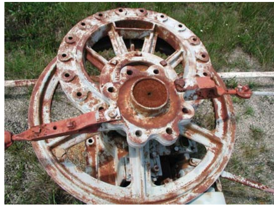
Figure 36. Detail of eccentric showing attachments for rod lines.
