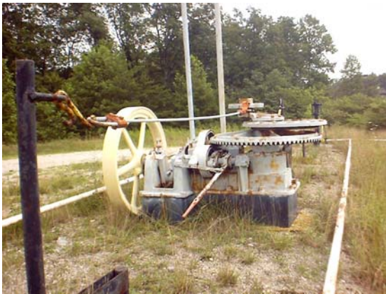
Figure 35. A Frick engine, a one cylinder, natural gas powered engine commonly used to provide power to pump multiple wells. The eccentric (the flat, toothed wheel to right) alternately pushed and pulled rod lines.
