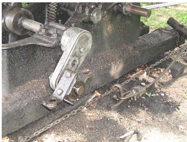
Figure 31. Pitman assembly. Detail of pitman assembly showing hook (hanging on chain) at the end of the pump drive cable and the eyelets (on the pitman) used to "hook up" wells.
