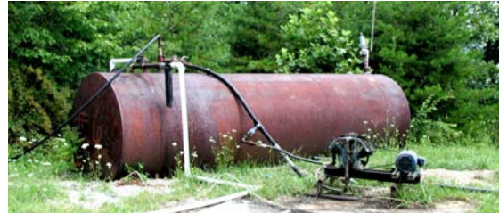
Figure 39. Generator and gas separator tank for power generation from produced natural gas.
