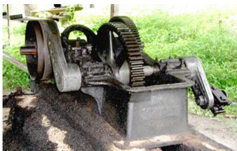
Figure 30. Gear box. Gearbox used to drive cable to pump producing wells. Belt on pulley to left is connected to drive shaft from the shed. The "pitman" on the right is used to convert rotational motion to the back and forth reciprocating motion required to pump wells.
