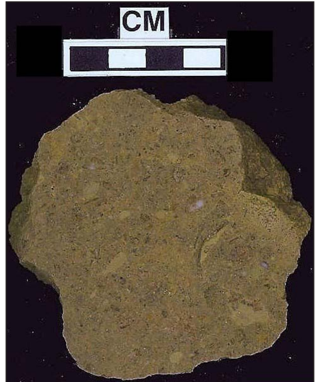
Figure 16. Polished slab of the Silurian Brassfield Formation, which is slightly phosphatic and glauconitic, showing crinoid, bryozoan, and other fragments in a greenish-yellow dolomite.
