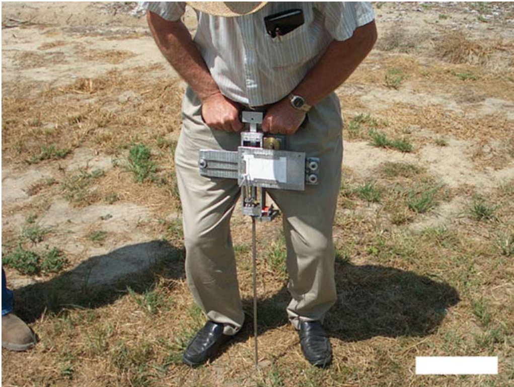
Using a penetrometer to check compaction.
