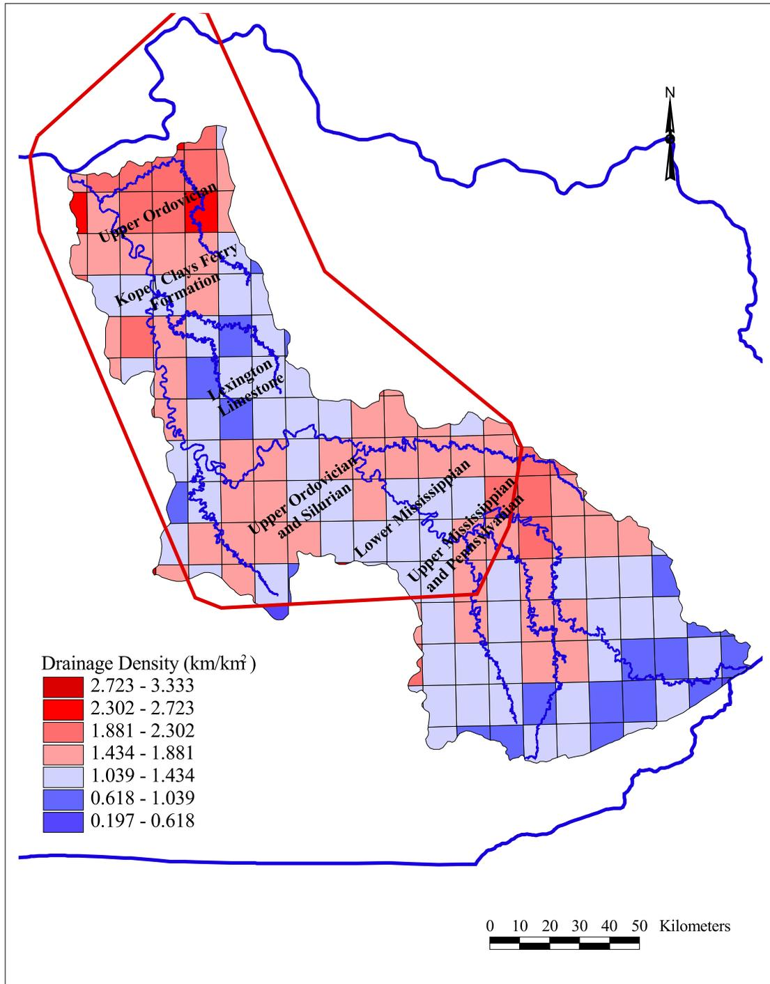
Figure 23. Drainage density for 7.5-minute quadrangles in the Kentucky River basin. The mean drainage density for the entire basin is approximately 1.434. General ages of bedrock shown by text; refer to Figure 4 for detailed bedrock geology.
