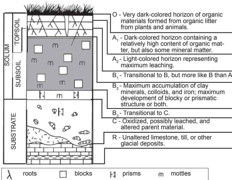
Figure 54. Soil terminology and horizons. Adapted from Aller (1982, Fig. 1). Reprinted with the permission of the Ohio Department of Health.
