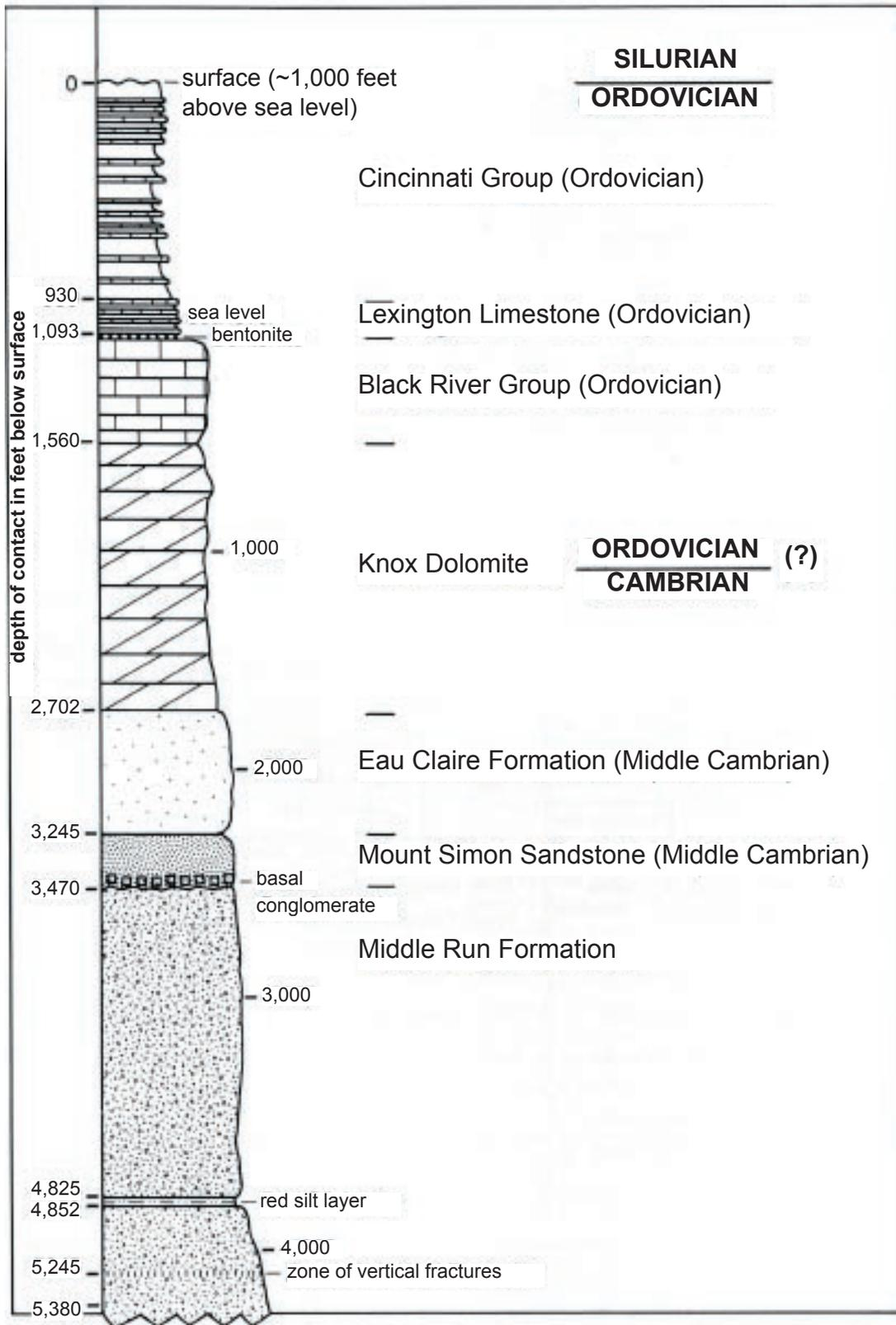
Figure 17. Geologic section encountered by the deep continuous core (DGS 2726) drilled in 1988 in northern Warren County by the Ohio Division of Geological Survey (Wolfe and others, 1989). Reprinted with the permission of the Society of Exploration Geophysicists.
