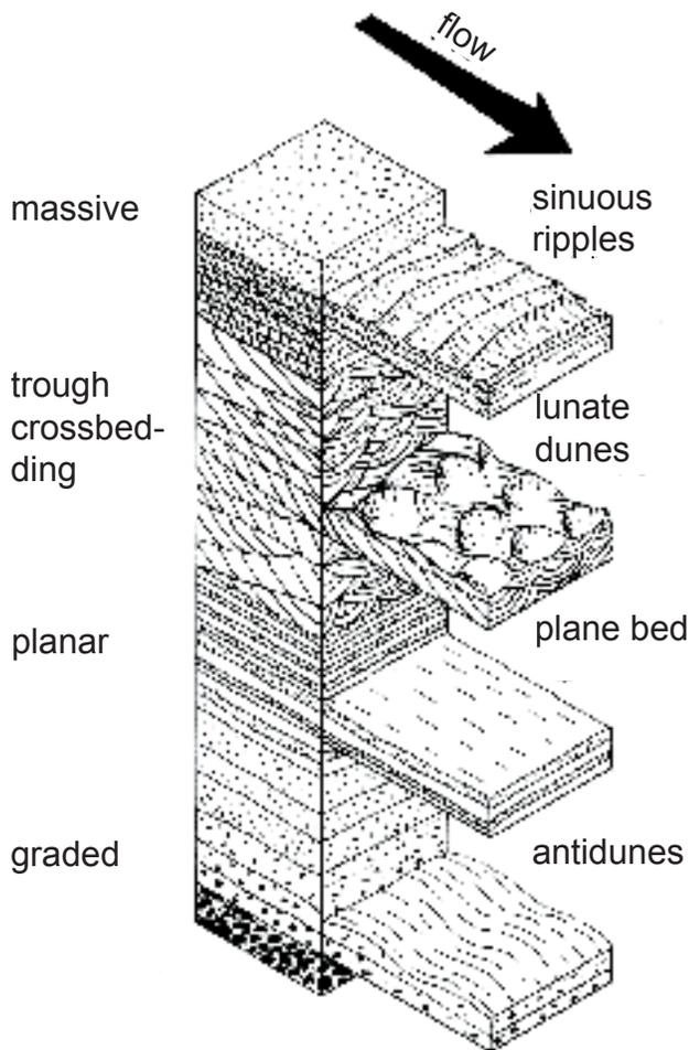
Figure 42. Typical sedimentary structures and their vertical sequence in fluvial deposits. Modified from Shelby (1985, Fig. 9.11). Reprinted with the permission of Oxford University Press.
