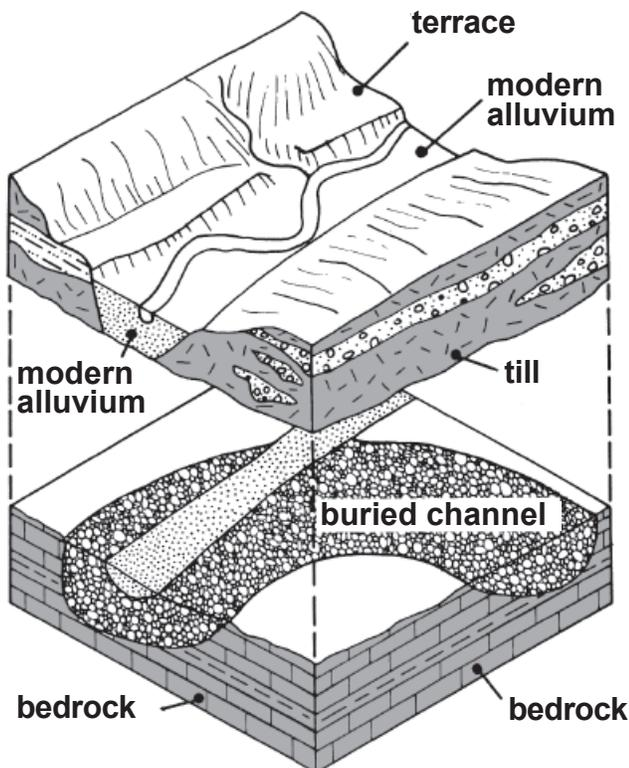
Figure 75. Idealized block diagram of recharge of gravel aquifer by a stream and gravel fill in an abandoned channel (Rosenshein, 1988, Fig. 4). Reprinted with the permission of the Geological Society of America.
