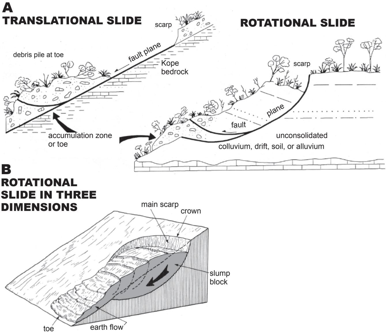
Figure 61. Definition diagrams for the principal types of landslides in the Cincinnati area. (A) Two principal types seen in cross section. (B) Block diagram of a rotational landslide (Bloom, 2004, Fig. 8-10). Reprinted with the permission of Waveland Press.
