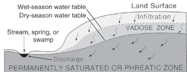
Figure 74. Definition diagram for infiltration and position of water table. Note how water table intersects the surface at a stream.
