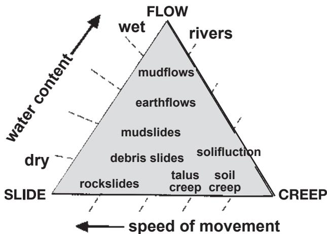
Figure 55. Mass-wasting triangle for controlling factors and nomenclature of mass movements (after Nuhfer and others, 1993). Reprinted with the permission of the American Institute of Professional Geologists.
