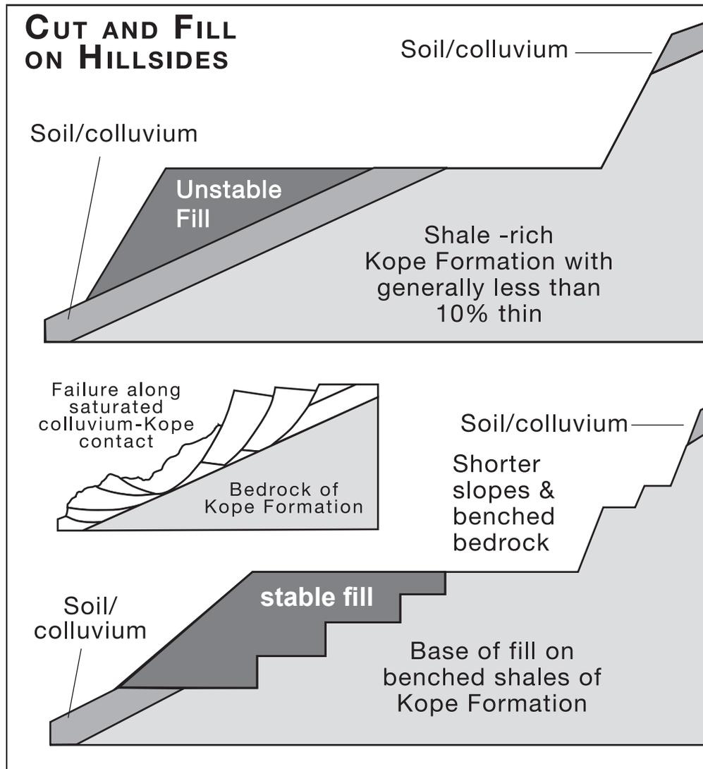
Figure 80. Benching a hillside underlain by shale needs special care, because shales readily generate colluvium in wet climates. Everywhere fill is placed on a hillside, failure is likely unless special precautions are taken.
