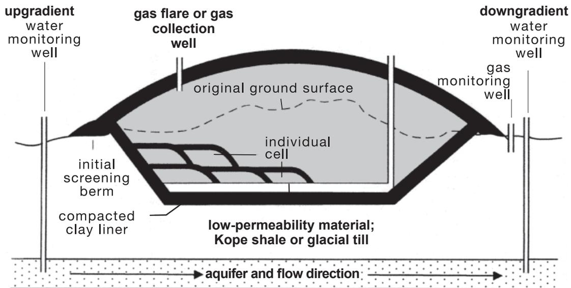
Figure 83. Diagrammatic cross section of a landfill. Redrawn from Aughenbaugh (1990, Fig. 1). Reprinted with the permission of Springer-Verlag Publishers.
