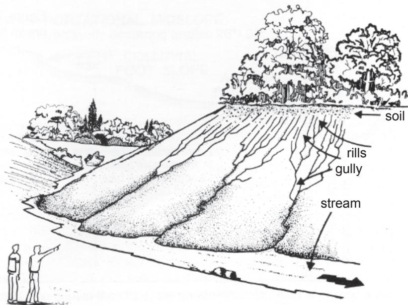
Figure 69. Rills and gulleys on a bare slope (redrawn from the Soil Conservation Service, undated, Fig. 3-1).
