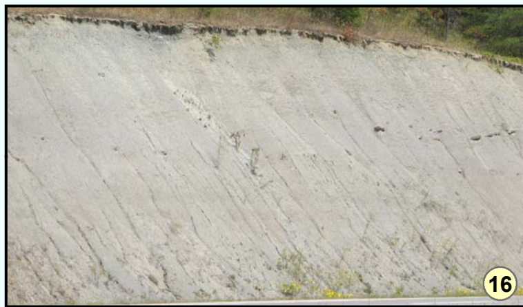
Mile 135.4: Greenish gray shale of the Nancy Member of the Borden Formation (Mbn) has potential for use in manufacturing drain and structural tiles; may contain ironstone concretions.
