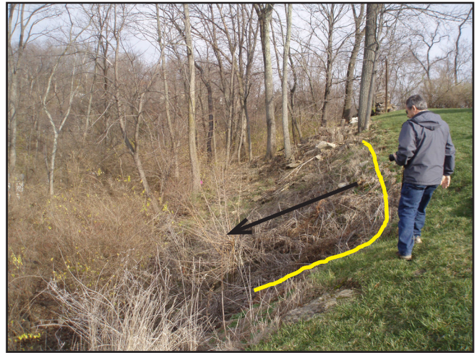
Figure 14. A scarp (outlined in yellow) from a recent landslide. Identification of offsets like this using LiDAR can flag these areas as highly susceptible to future failure.
