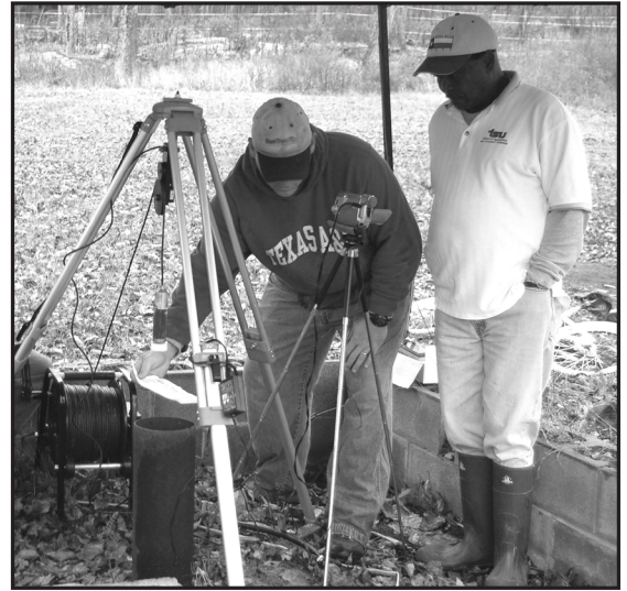
Glynn Beck trains Sam Dennis of Tennessee State University on use of a video camera in a domestic well in Murfreesboro, Tenn.
