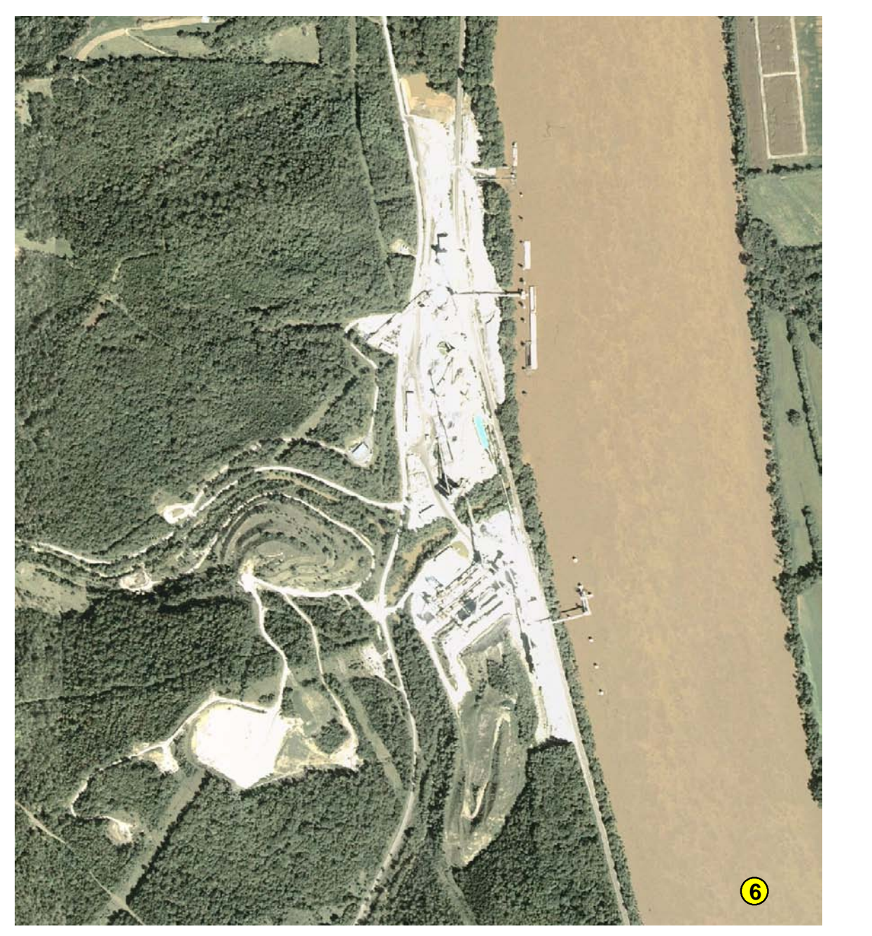
Carum Lime produces 1.4 million tons per year of high-calcium lime for power-plant scrubbers and the steel industry from its 600-foot-deep slope mine on the Ohio River. Aerial photo (2004) by the U.S. Department of Agriculture, Farm Services Administration, National Agricultural Imagery Program.
