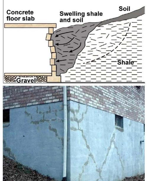
Some shales, and the soils derived from them, swell when exposed to water or air. These swelling shales and soils can have severe impacts on building foundations and other structures (e.g., bridges, dams, roads). Photograph by John Kiefer, Kentucky Geological
