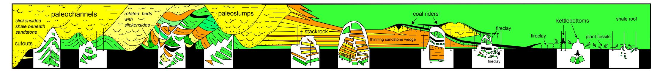
Figure 8. Schematic diagram showing the types of lateral variation seen in roof rocks, and inherent mining obstacles associated with each, above the Lower Elkhorn coal bed. Rates of variation are variable, which is why no scale is inferred.
