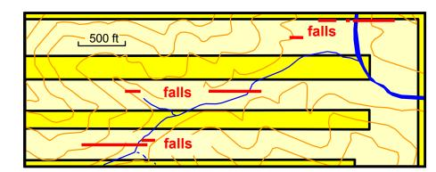
Figure 7. Roof falls (red) beneath low cover in an underground mine (light yellow). Blue lines are streams and orange lines are surface contours (after Greb and Popp, 1999, Fig. 13A).
