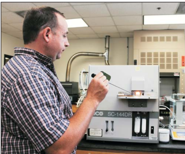
Laboratory Manager Jason Backus places samples in a sulfur and carbon analyzer that combusts the samples at 1,400 degrees Celsius.
