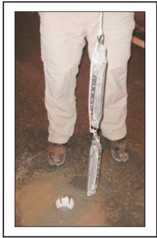
Baskets of limestone were installed by the Water Resources Section in Cumberland Gap Tunnel monitoring wells to monitor dissolution of the rock.
