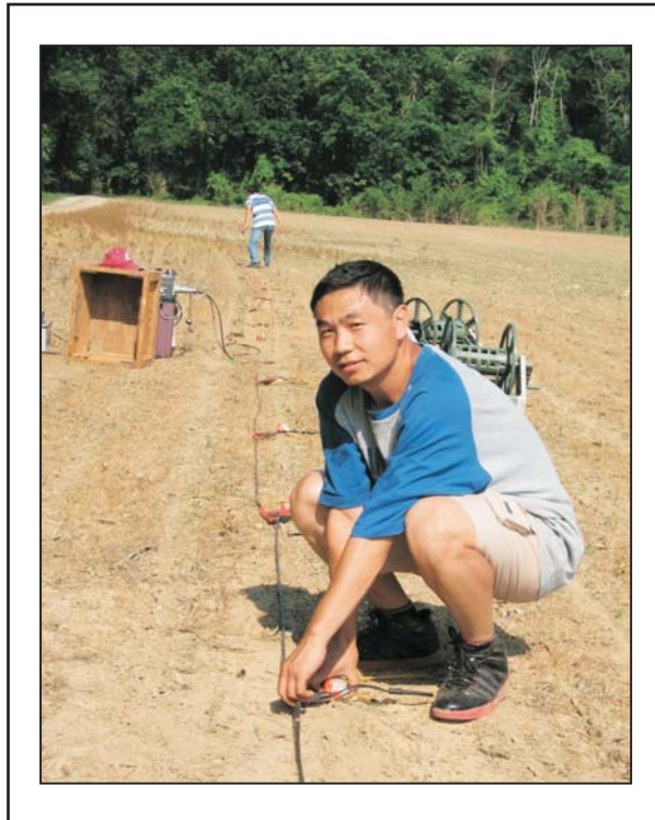
Visiting scholar Shunhua Xu couples a shear-wave geophone to the ground for a seismic velocity sounding near the Ohio River in McCracken County in a USGS-funded collaborative project between KGS and the University of Memphis.
