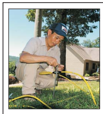
Junfeng Zhu of the Water Resources Section sets up electrical-resistivity equipment to detect groundwater in Burnside, Ky., where ground movement may be damaging nearby houses. He has used this equipment in other projects, including the Cane Run watershed project.
