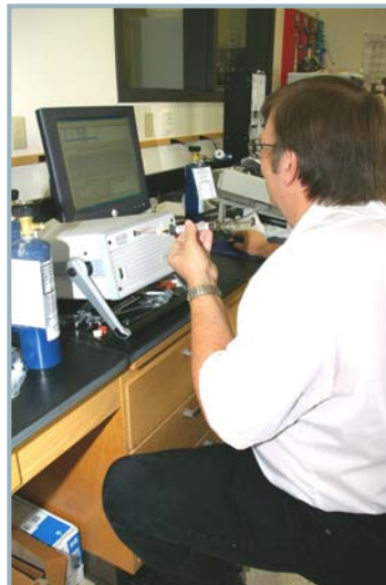
Steve Mock injects a sample into a gas chromatography instrument in the lab to determine its properties.
