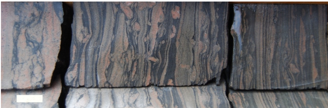
Figure 3.60. Contorted bedding and deformed vertical burrow at 3122 ft in Unit 6. Top is upper left in photo. Scale bar is 1 cm. Core shown wet to enhance bedding contrast.
