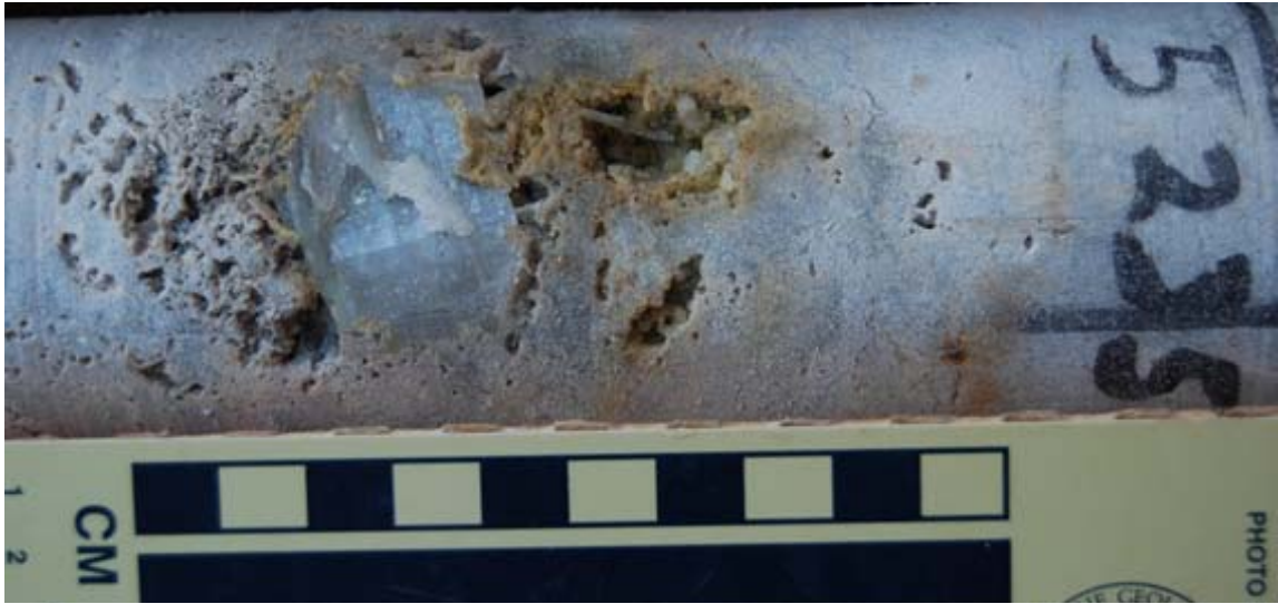
Figure 3.70. Vuggy porosity in Unit 4 dolomite at 5235.00 ft deep. Top of core is to right.
