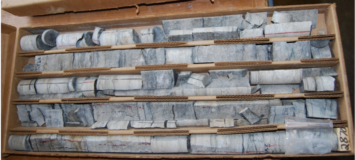
Figure 3.55. Interbedded sandstone, siltstone and shale at the top of Unit 4, in the Warren County well from depths of 2860 to 2870 ft. Top is upper left in photograph. Each core row is two ft long.
