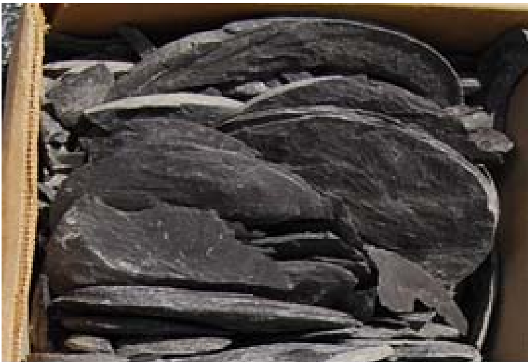
Figure 3.31. Typical brittle, broken shale in Unit 4 in the DuPont No. 1 WAD fee well. Core width is four inches.
