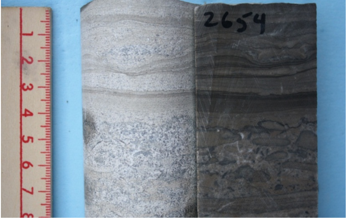
Figure 3.48. Sharp-based flat-pebble conglomerate above laminated dolomitic limestone, interbedded with laminated dolomitic limestone and shale at 2654 ft depth. Wet and dry core halves are shown. Ruler scale in cm.
