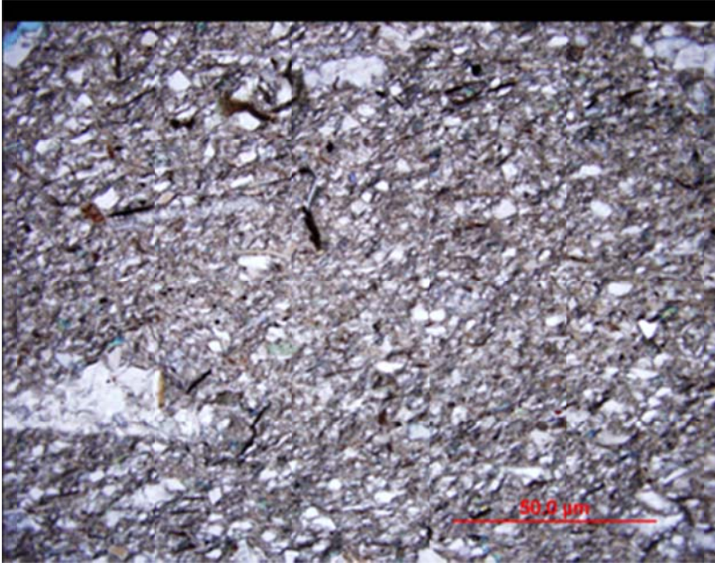
Figure 3.43. Photomicrograph of silty shale from 2839 ft deep from Unit 1. Biotites are dark brown. Note vertically aligned biotites and finer matrix in center of the photomicrograph, which may represent a burrow. 100x magnification with cross polars.
