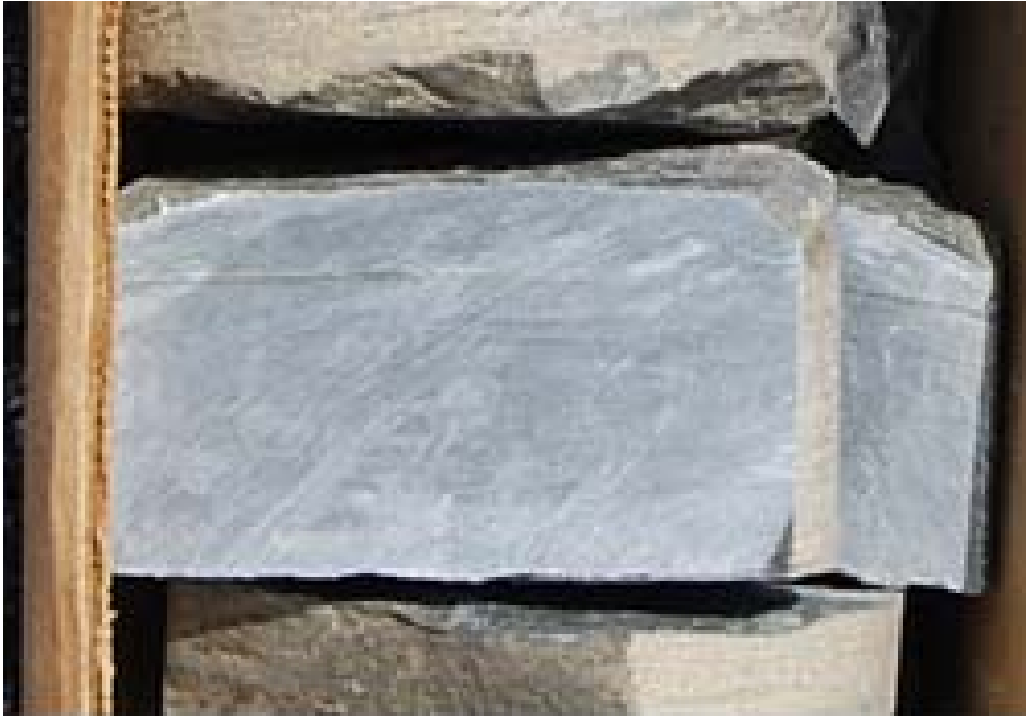
Figure 3.30. Laminated siltstone in Unit 4 in the DuPont No. 1 WAD fee well. Core width is four inches.
