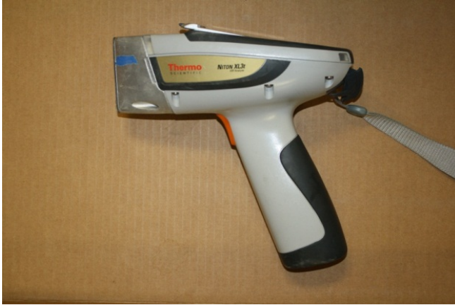
Figure 2.1. A Thermo Scientific Niton XL3 portable XRF device was used to analyze shale chemistry in the core. Data on major, minor, and trace elements were collected.
