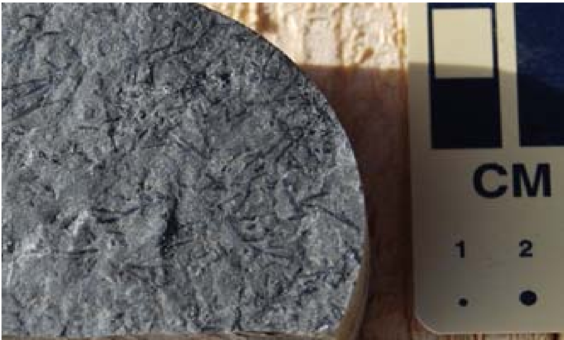
Figure 3.65. Graptolite fragments in lower part of Unit 1 shale at 5062.50 ft deep.
