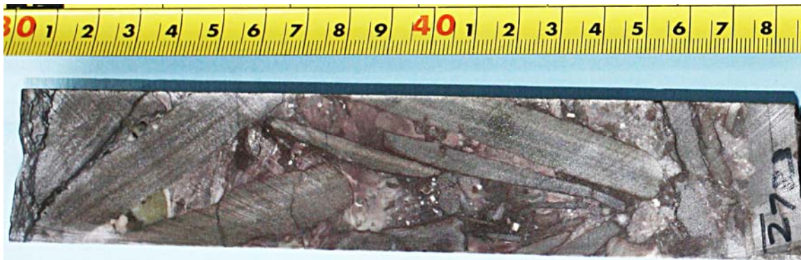
Figure 3.54. Flat-pebble conglomerate comprised of large clasts, with red to pink iron (?) staining at 2783 ft. Top is to the left. Ruler scale in cm.
