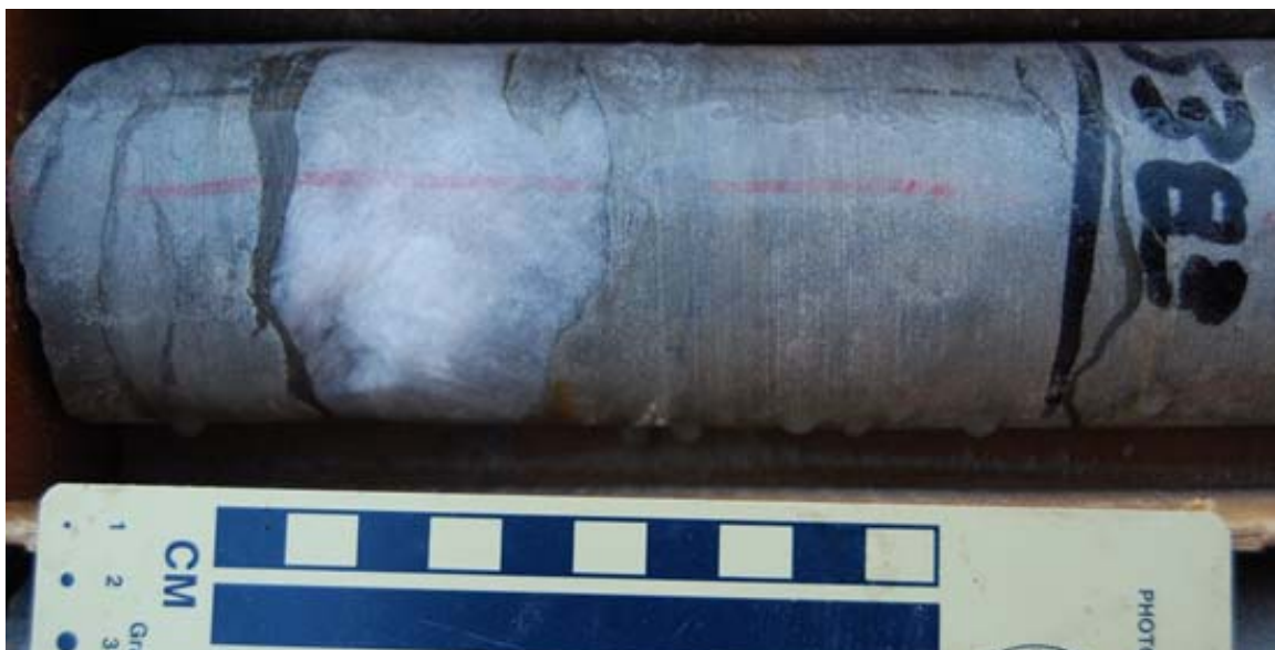
Figure 3.71. Irregular anhydrite bed (white and light blue) in Unit 4 dolomite at 5383.5 ft. Top of core to right.
