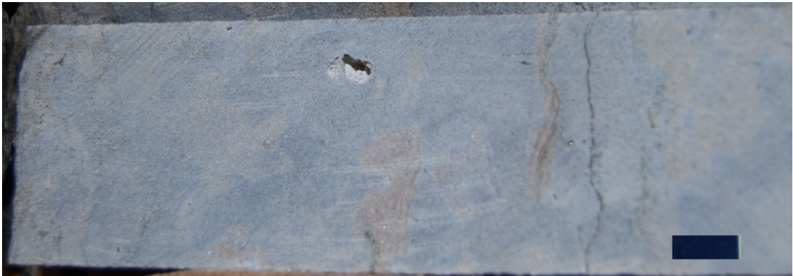
Figure 3.58. Small, isolated vug in gray contorted, partially dolomitic, siltstone at depth of 3079.5 ft. Scale bar is 1 cm. Top is upper left in photo.
