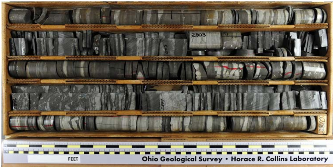
Figure 3.53. Example of interbedded siltstones and shales in Unit 3 in the Warren County well from 2800 to 2810 ft. Top is upper left in photograph. Core shown wet to enhance bedding.
