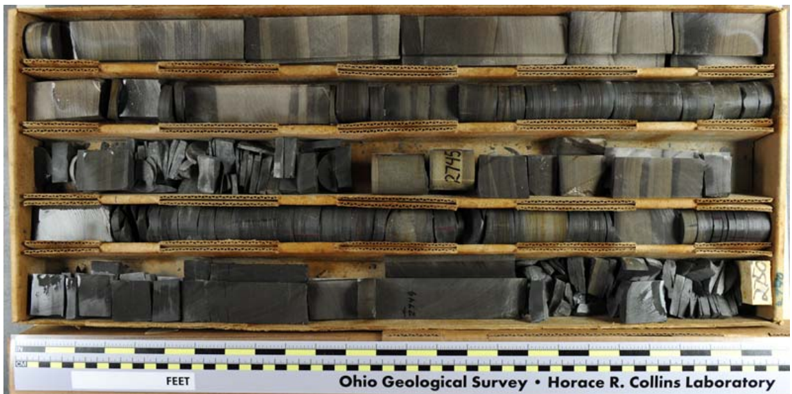
Figure 3.51. Example of interbedded shale (dark) and siltstone (light) from lower in Unit 2, at depths of 2740 to 2750 ft. Top is upper left in photograph. Core shown wet to enhance bedding contrast.
