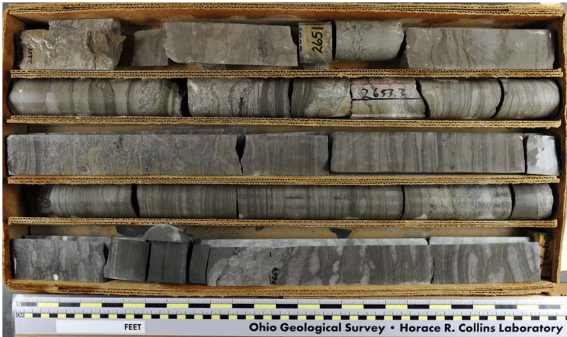
Figure 3.47. Unit 1 dolomites and interbedded shaly dolomites and shales in the Warren County well at depths of 2670 to 2680 ft deep. Top is upper left in photograph.
