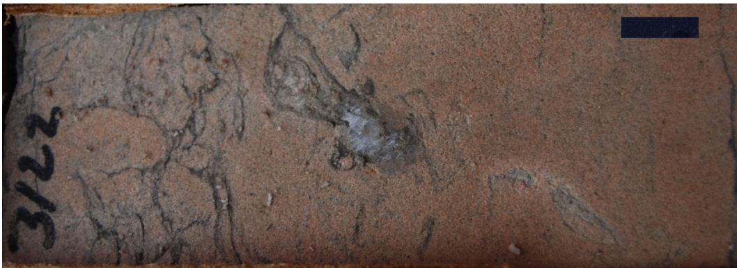
Figure 3.60. Contorted bedding and deformed vertical burrow at 3122 ft in Unit 6. Top is upper left in photo. Scale bar is 1 cm. Core shown wet to enhance bedding contrast.
