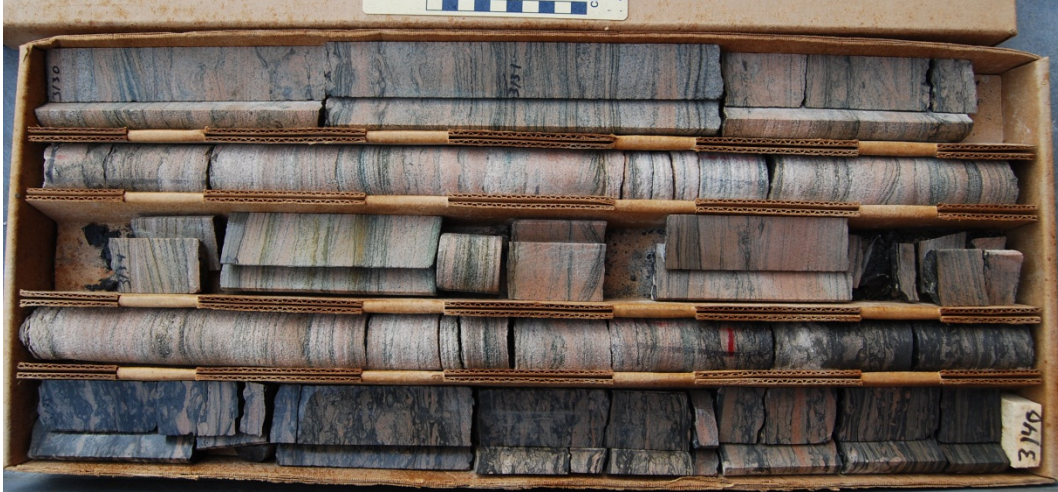
Figure 3.59. Sandstone and interbedded shale in Unit 6 from 3130 to 3140 ft. Top is upper left in photo. Scale in cm. Core shown wet to enhance bedding contrast. Note pink color in some sandstones.
