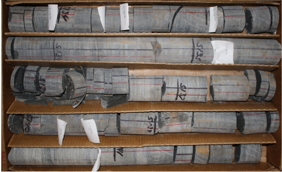
Figure 3.68. Unit 2 shales from 5133 to 5142 ft deep. Top is upper right. Each core row is 2 feet in length. Paper slips mark position of fossils in the core.
