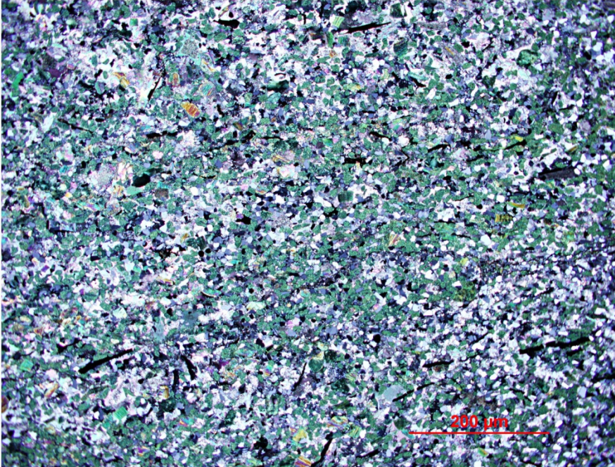
Figure 3.34. Photomicrograph of bioturbated siltstone from 4859 ft deep in Unit 1. Note abundant glauconite grains. 20x magnification with cross polars.
