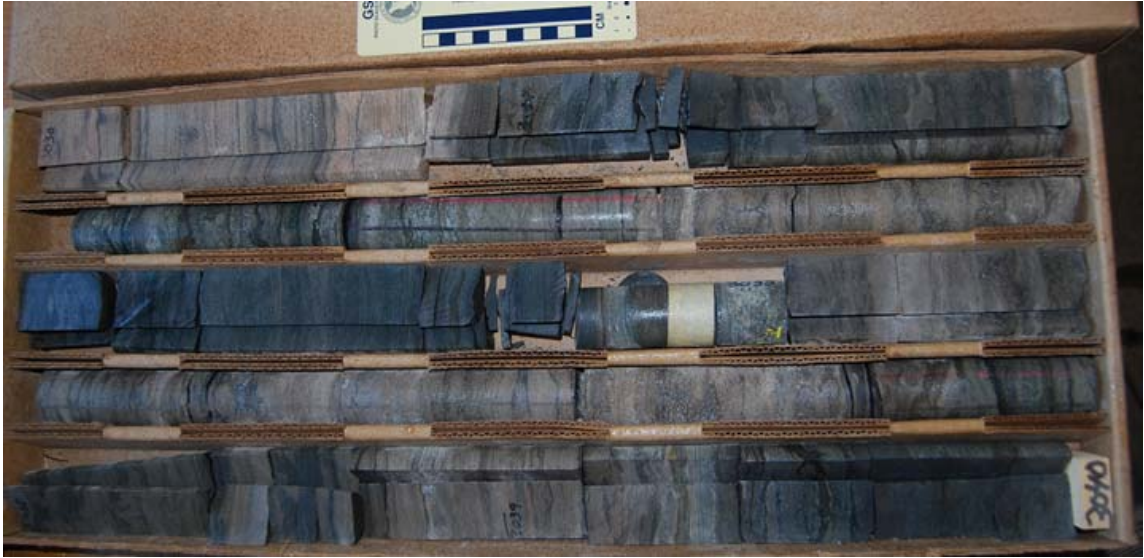
Figure 3.57. Interbedded siltstones and shales in Unit 5 from 3030 to 3040 ft. Top is upper left in photo. Scale in cm. Core shown wet to enhance bedding. Note pink color in some siltstones.
