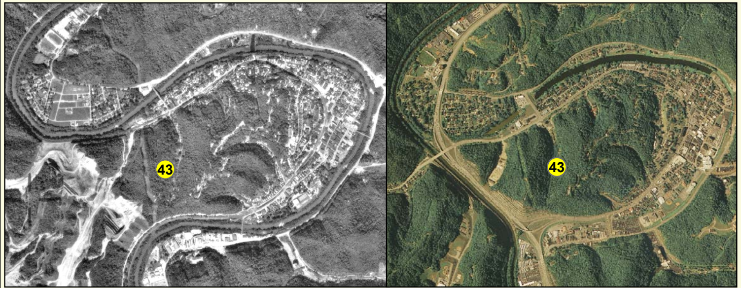
Mile 24.3–23.8: The Pikeville Cut-Through controls flooding by rerouting Levisa Fork away from the oxbow that encircles Pikeville. The 1974 photo at left shows conditions before the cut-through compared with conditions after the cut-through in 2006 (photos from U.S. Department of Agriculture). The cut-through is 1,300 feet wide, 3,700 feet long, and 523 feet deep, and is second only to the Panama Canal. Extensive development has taken place in the 393 acres created by the cut-through.
