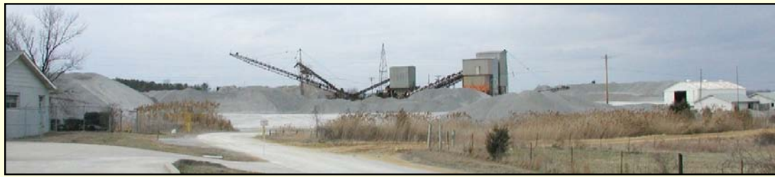
Ragland Quarry, a mile west of Leitchfield off of Ky. 54, produces 300,000 tons of crushed stone, asphalt, and lime a year from the Glen Dean Limestone (Mgd) and Haney Limestone Member of the Golconda Formation (Mgh).
