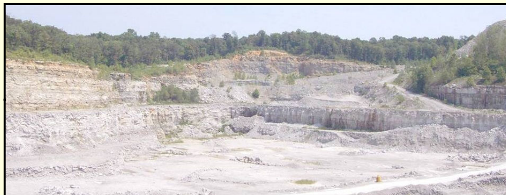
Limestone is abundant in Caldwell County. The Princeton Quarry of the Rogers Group produces 800,000 tons of crushed stone each year from the Ste. Genevieve Limestone (Msg). The quarry, on the southeast side of Princeton off of Ky. 91, has been in operation since 1891. Photo by Glynn Beck, Kentucky Geological Survey.
