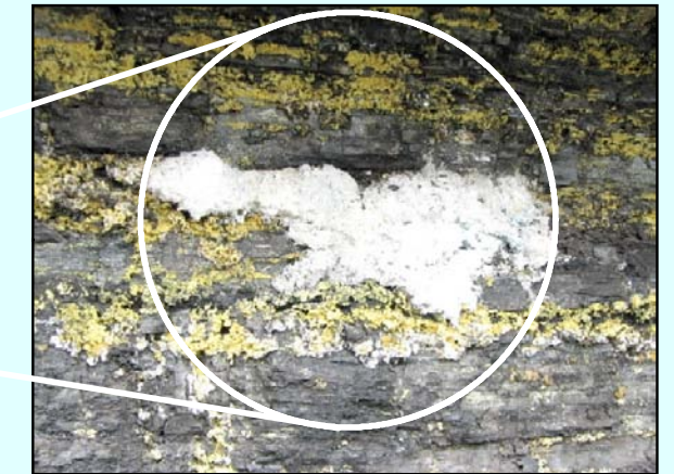
White and yellow sulfur precipitates from pyrite weathering in the coal.
