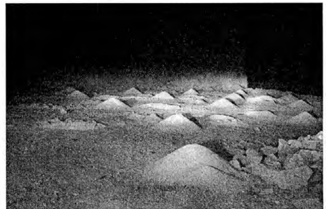
Figure 27. Floor of mine, drilled 16 feet deep.
