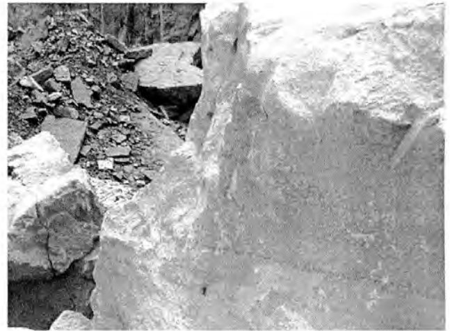
Figure 23. Stylolites present in limestone.
