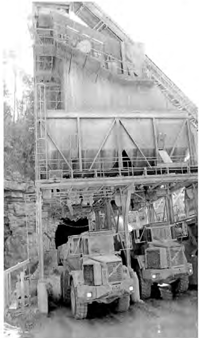
Figure 25. Trucks being loaded at load-out bins with finished product.
