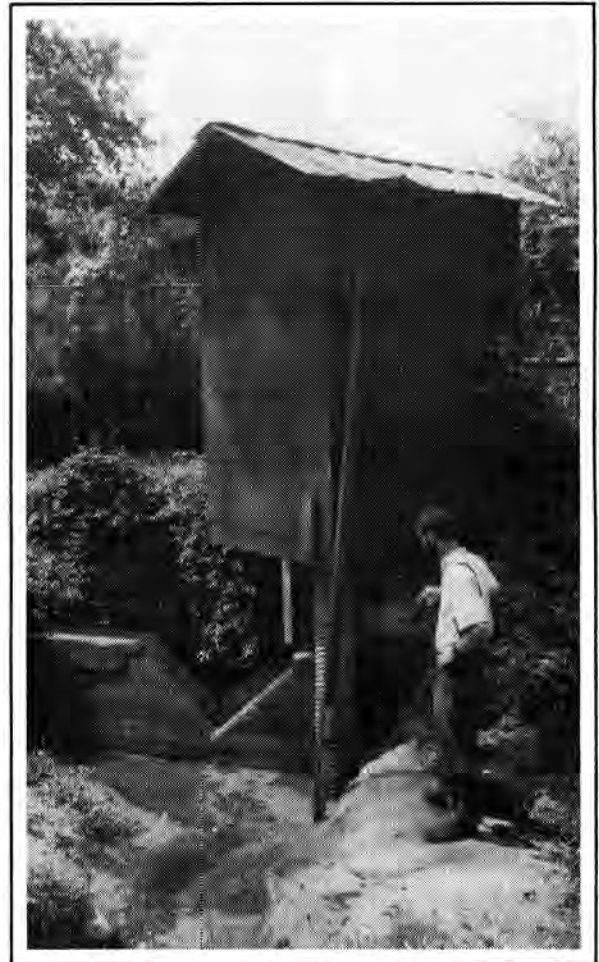
Figure 29. V-notch weir and recording instruments at the entrance to Bypass Cave (Stop 4).
