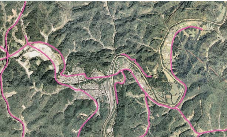
▲ This map of the Paintsville area, highlighting road segments with repetitive repair costs, is an example of the graphics KGS staff is creating to help the Transportation Cabinet track locations of high costs from geologic hazards.
