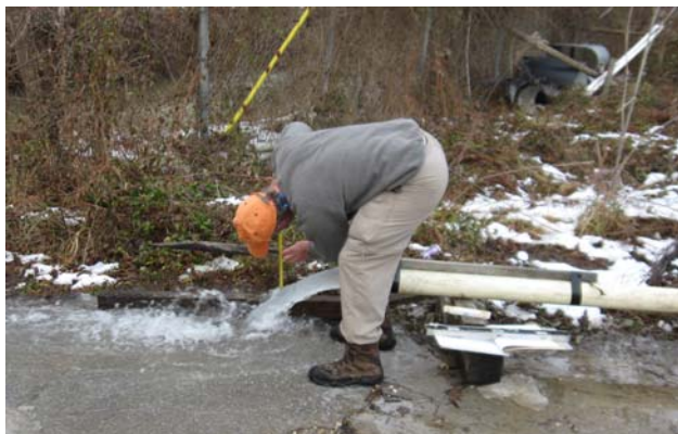
▲ Jim Dinger measures groundwater flow from a discharge pipe during a pumping test of a sandstone aquifer in Campton.
