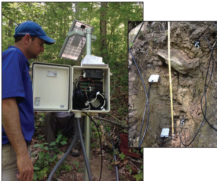
Matt Crawford sets up a monitoring station at a Kenton County landslide. Sensors buried at the top and bottom of the slide, monitor hydrologic conditions such as water content, electrical conductivity, and temperature.
