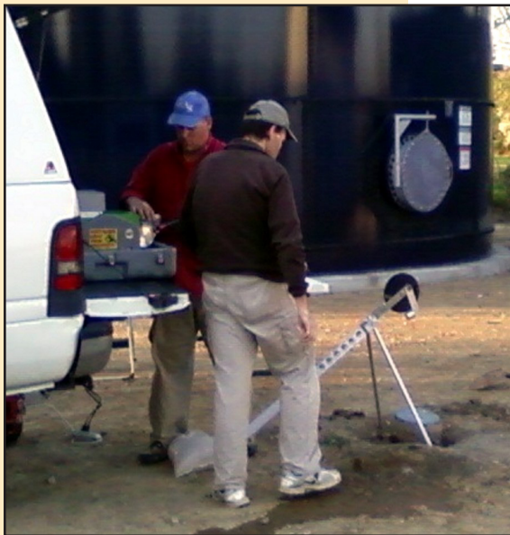
Glynn Beck and Steve Webb set up a downhole camera to inspect a well at White Plains in Hopkins County.
