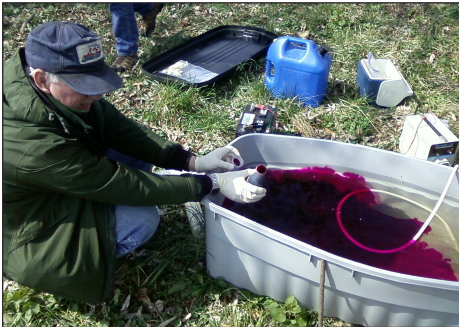
Jim Currens introduces premeasured nontoxic fluorescent Rhodamine WT dye into a tub of water to begin a tracer test at the Kentucky Horse Park in the Cane Run Basin.
